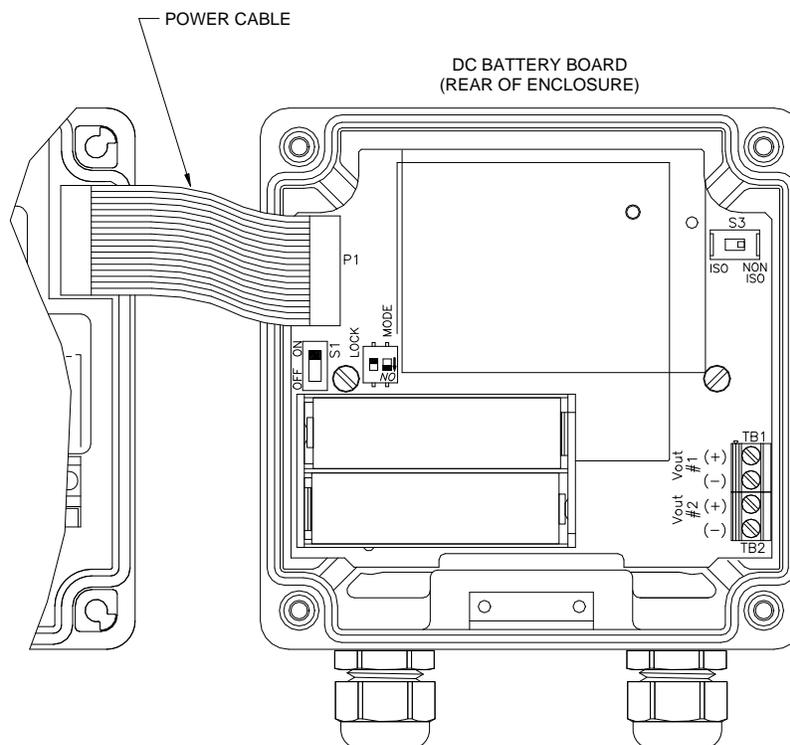
**Figure 5 - Battery Board Connections**
