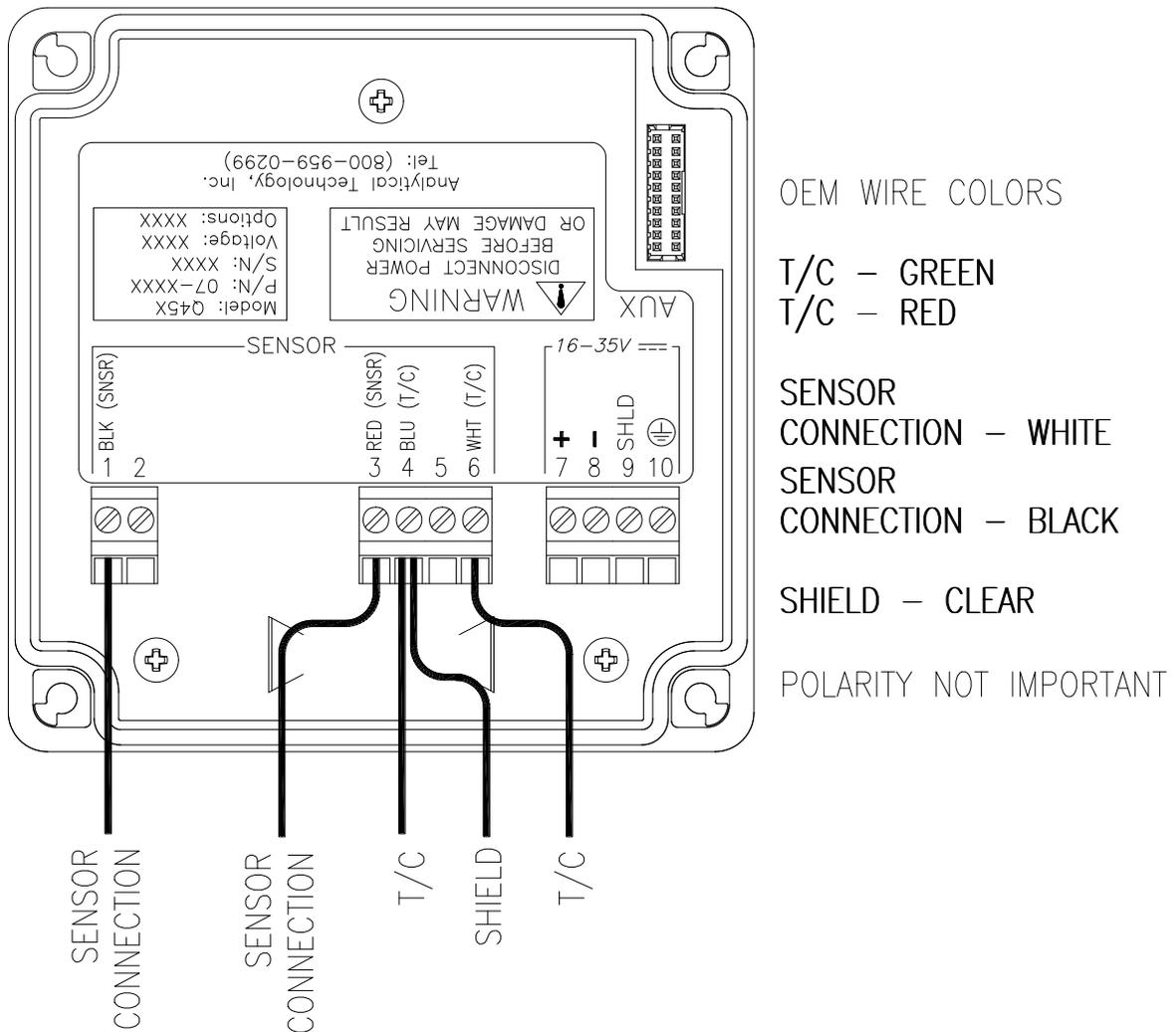
**Figure 4 - OEM Sensor Connections**
