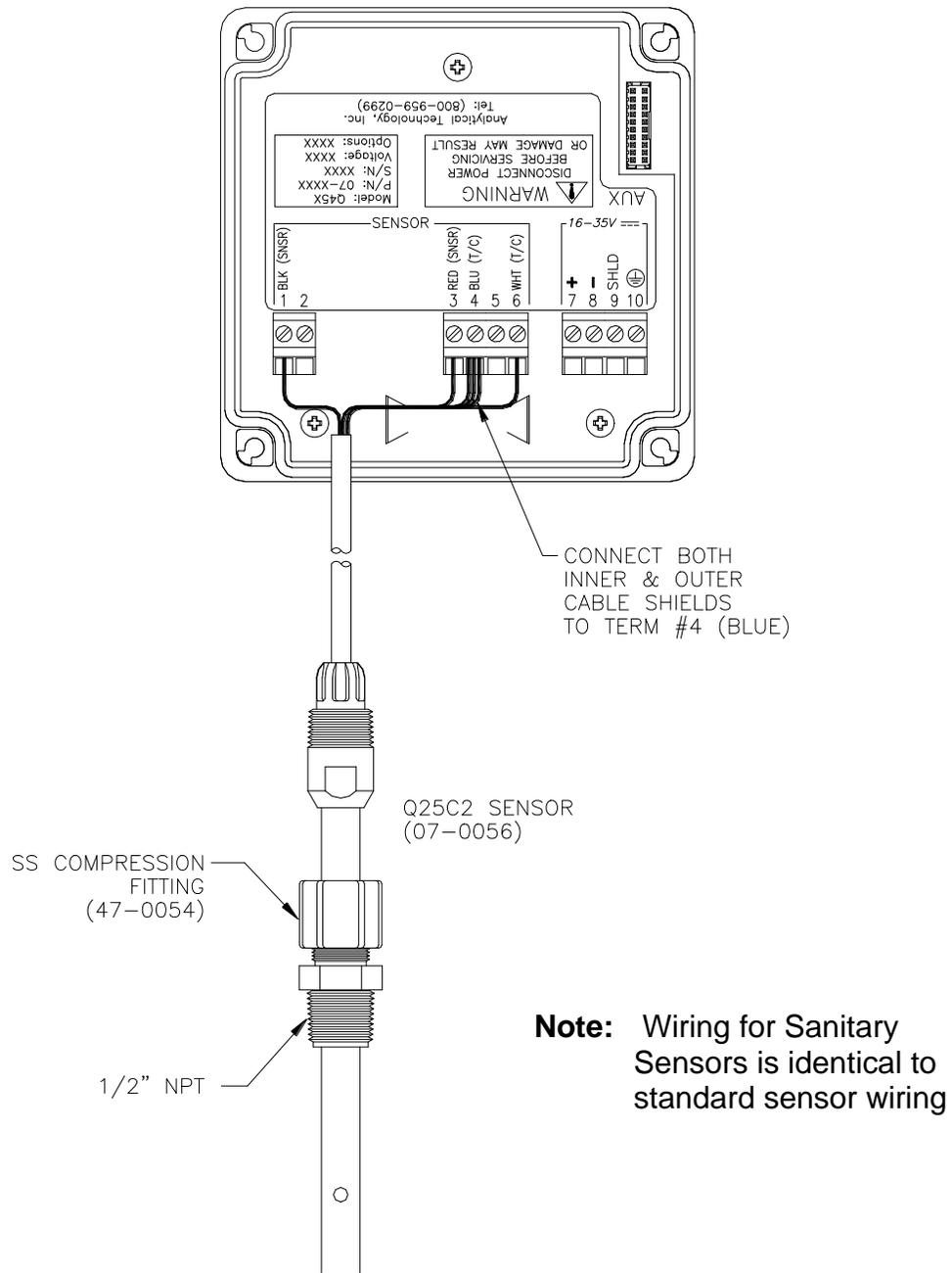
**Figure 3 - Sensor Connections**
