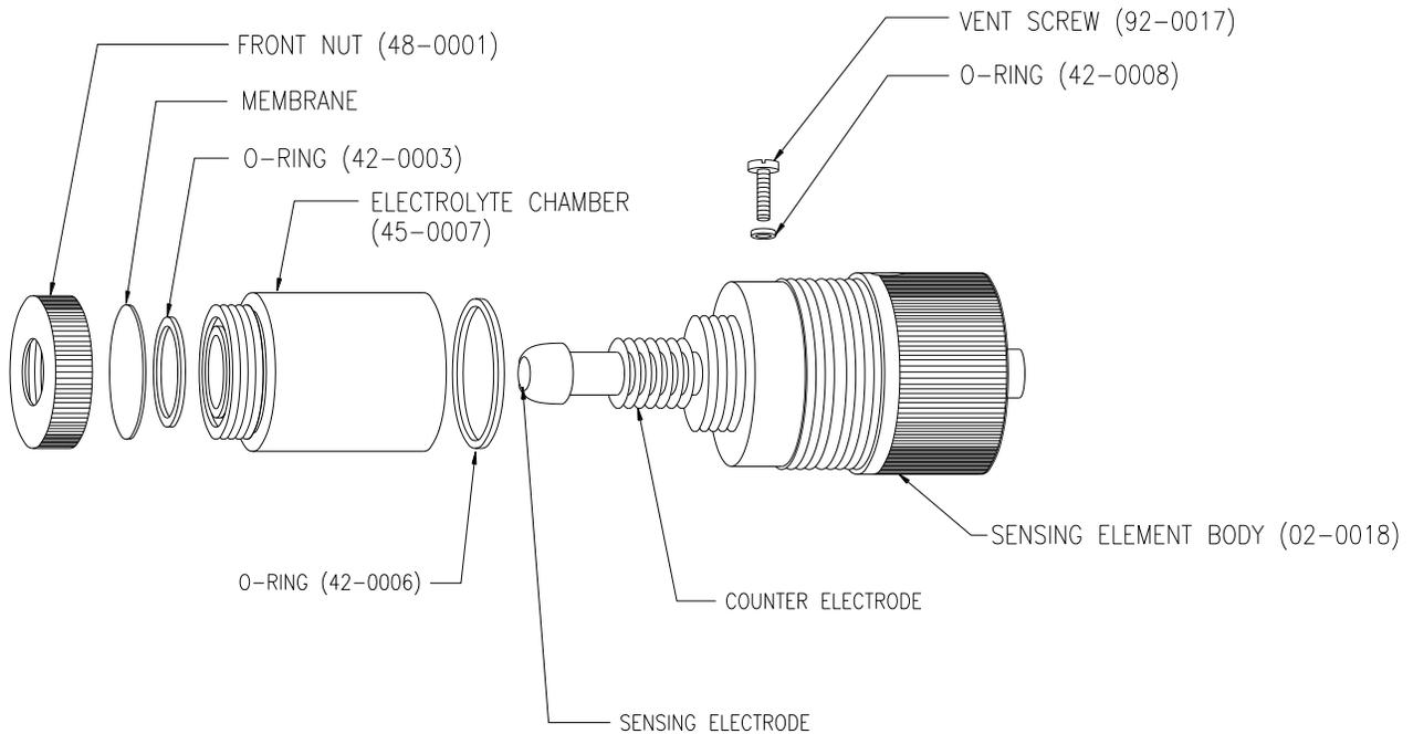
**Figure 6 - Ozone Sensor Assembly (ATI-0294)**
