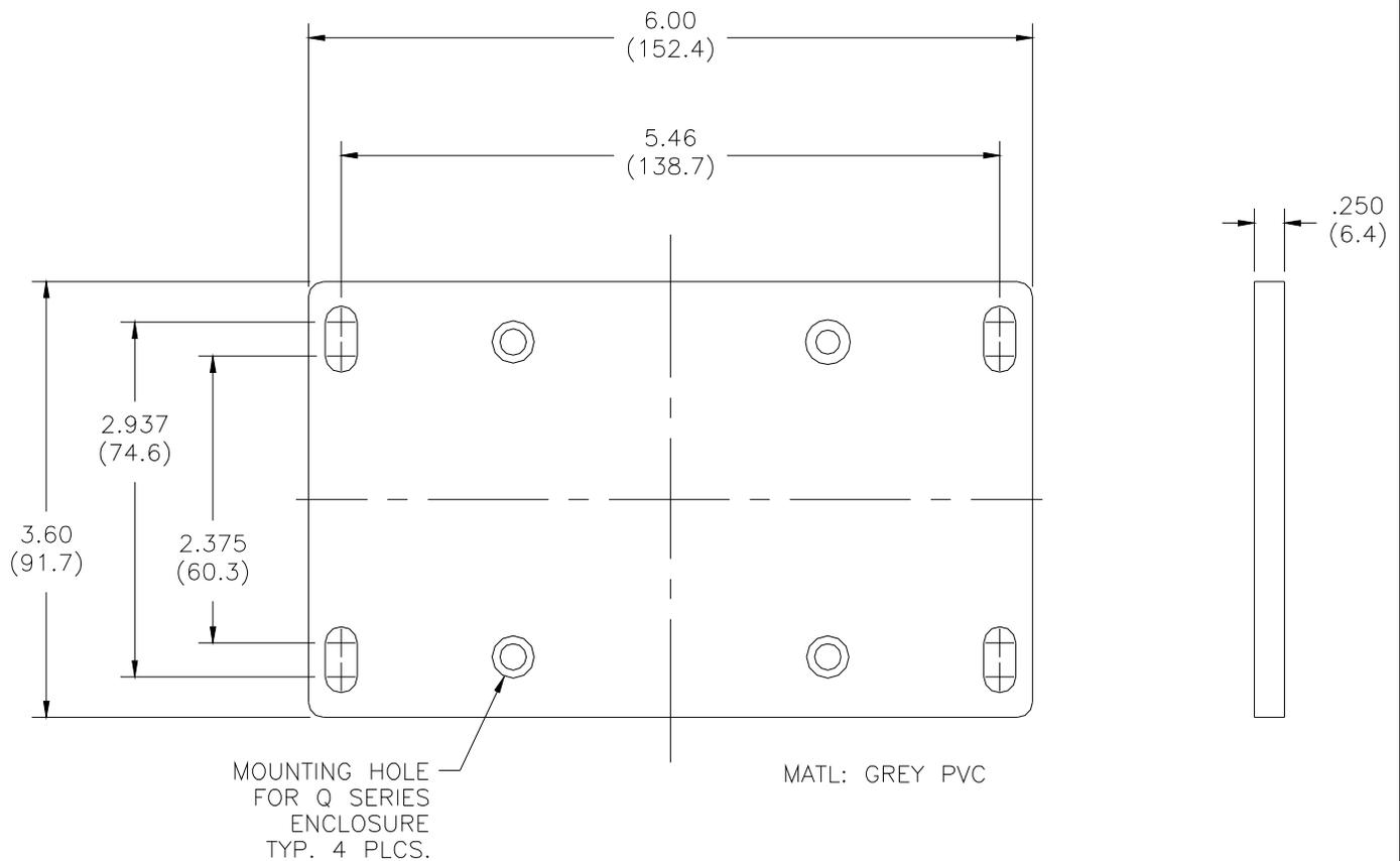
**Figure 5 - Wall or Pipe Mount Bracket**
