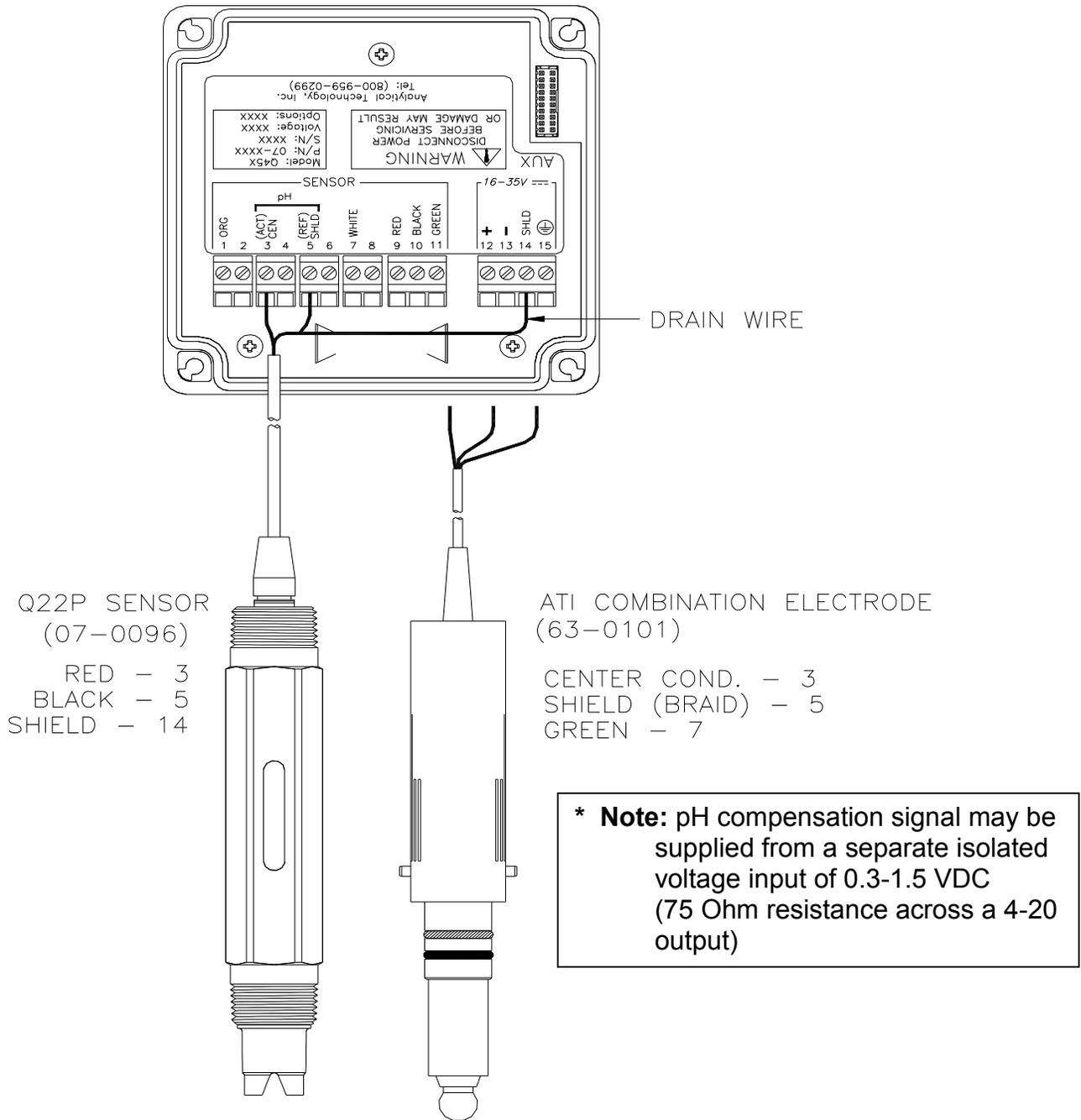
**Figure 15 - Optional pH Sensor Connection**
