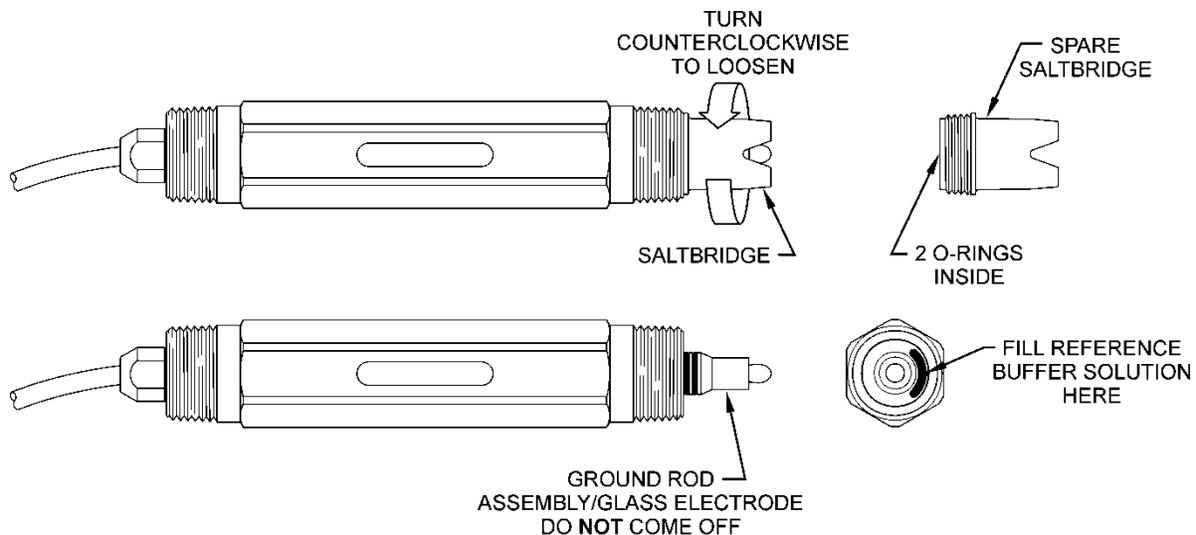
**Figure 23 - Replacing the Saltbridge and Reference Buffer**
