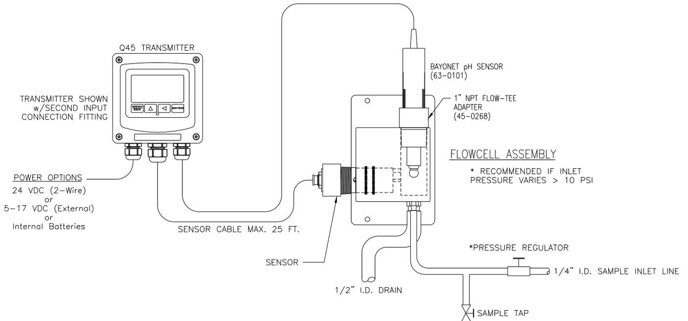
**Figure 2 - Monitoring System w/Bayonet style pH Sensor**
