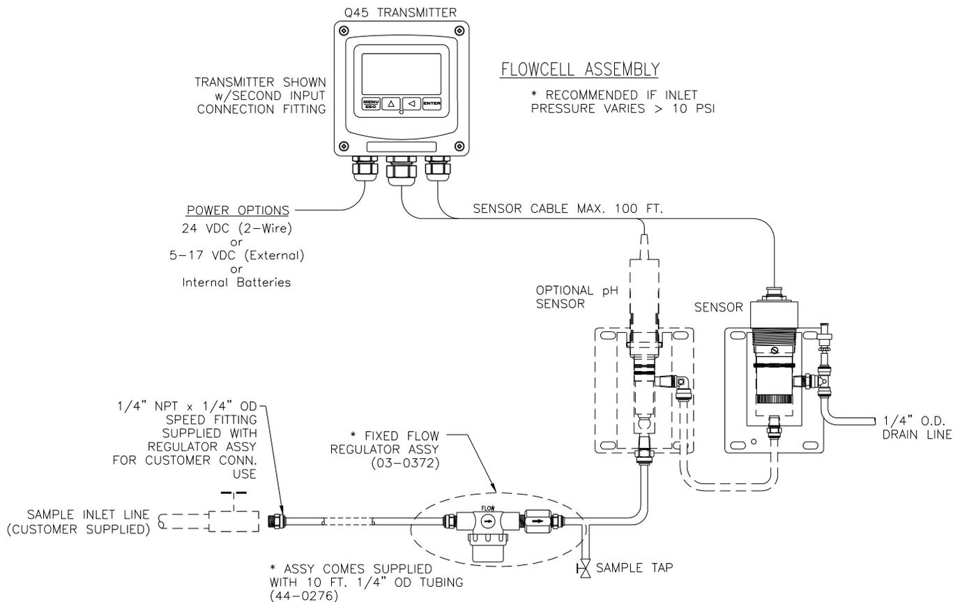
**Figure 3 - Sealed Flowcell Assemblies w/Flow Control**
