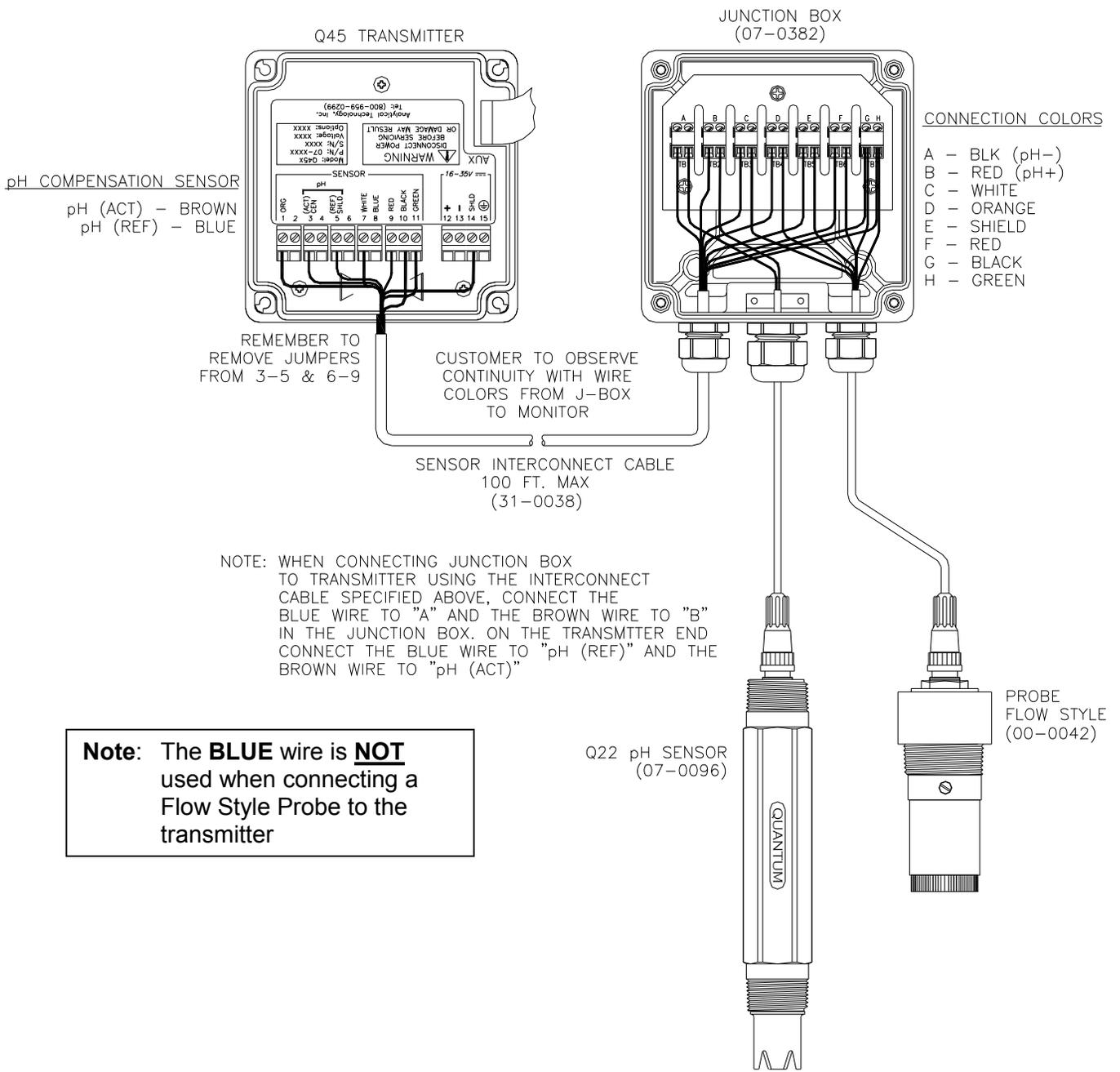
**Figure 16 - Optional pH Sensor Connection w/Junction Box**
