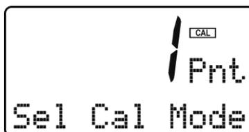
5. The system now begins acquiring data for the calibration value. As data is gathered, the units for pH and temperature may flash. Flashing units indicate that this parameter is unstable. The calibration data point acquisition will stop only when the data remains stable for a pre-determined amount of time. This can be overridden by pressing ENTER. If the data remains unstable for 10 minutes, the calibration will fail and the message **Cal Unstable** will be displayed.
