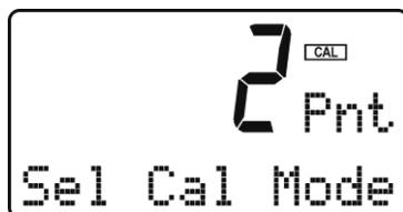
5. The display will prompt the user to place the sensor in the first mV solution and press ENTER. If the sensor has been placed into this solution already, once the temperature has stabilized, press ENTER to continue.
