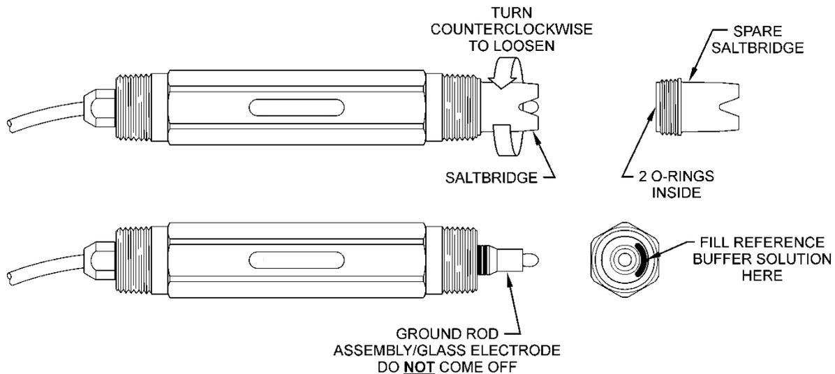
Figure 9 - Replacing the Saltbridge and Reference Buffer
