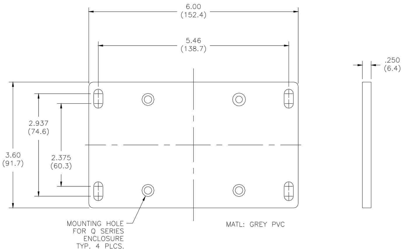
**Figure 2 - Wall or Pipe Mount Bracket**
