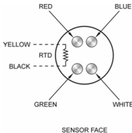
3. Verify that the sensor’s temperature element (Pt1000 RTD) is functioning properly by measuring the resistance between the sensor’s yellow and black wires. The nominal resistance value at 25°C is 1097 ohms. Use the following table as a guide to the approximate resistance value:
