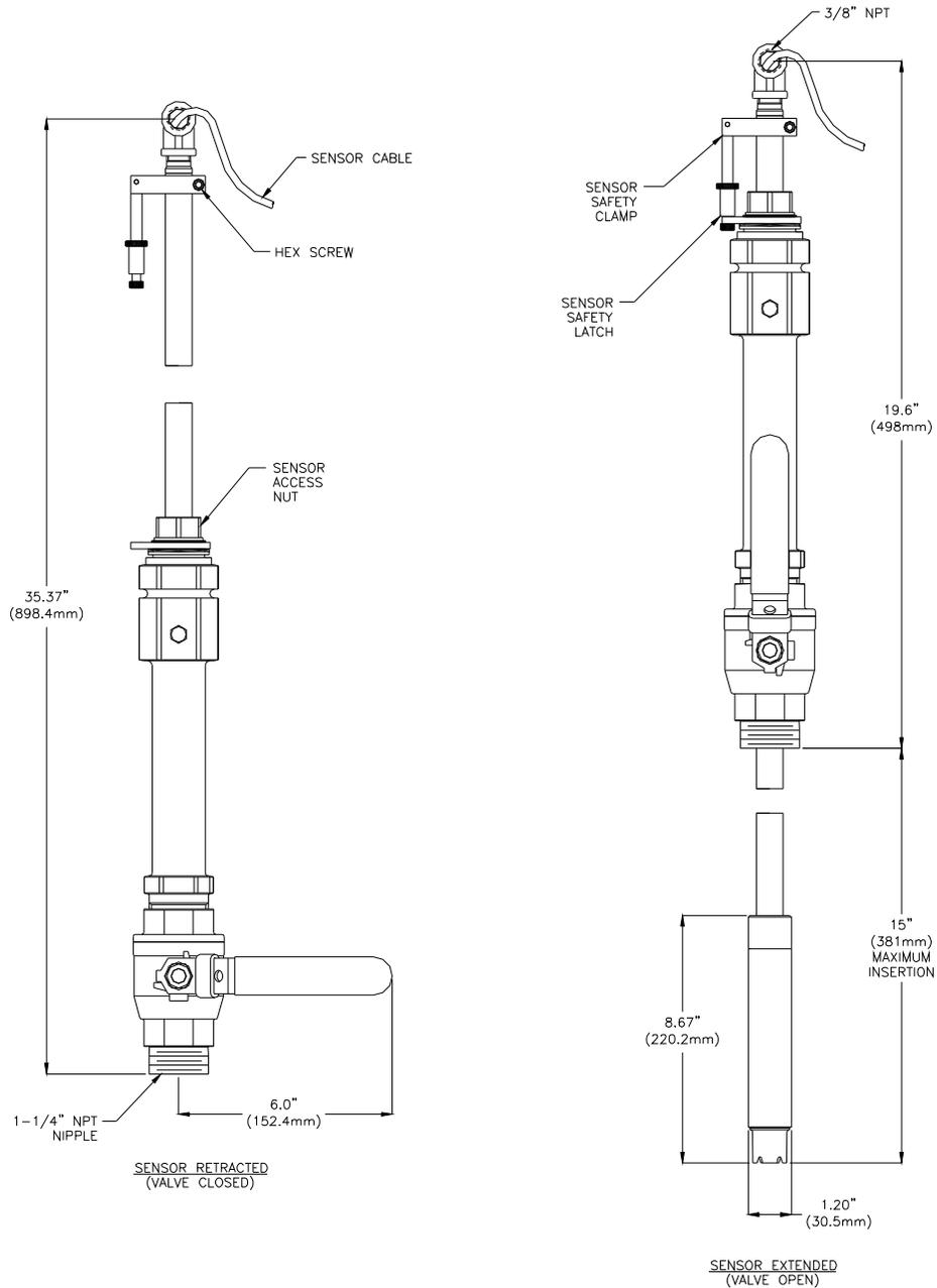
**Figure 12 - S.S. Sensor Insertion Mount**
