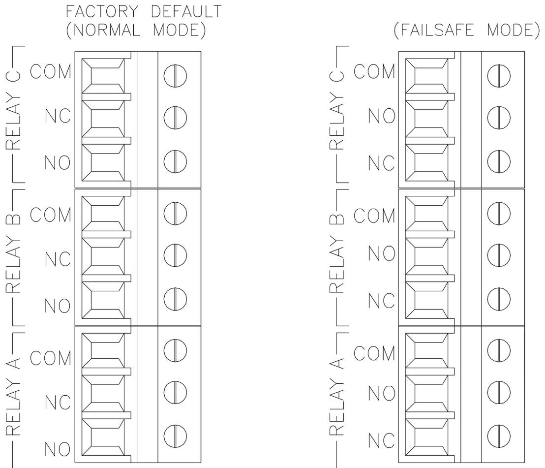
**Figure 15 - Relay Connections**
