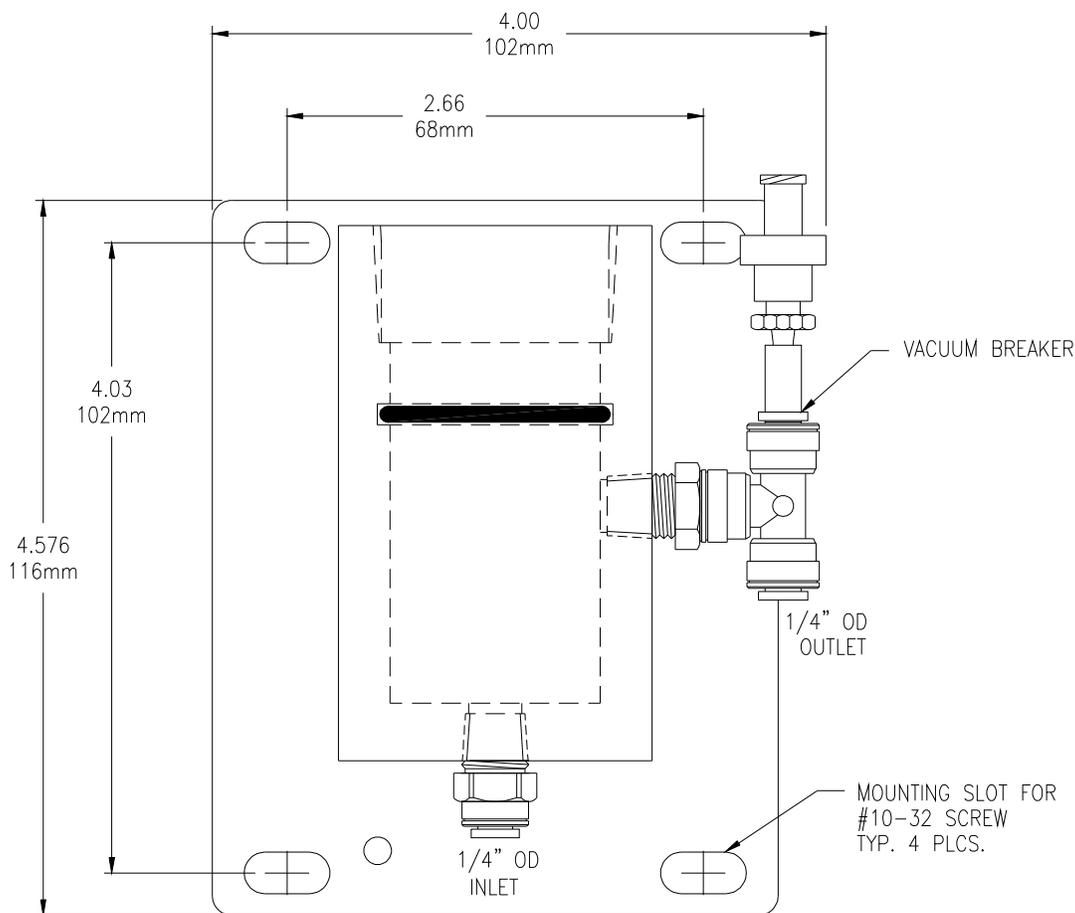
Figure 10 - Sealed Cl<sub>2</sub> Flowcell Details
