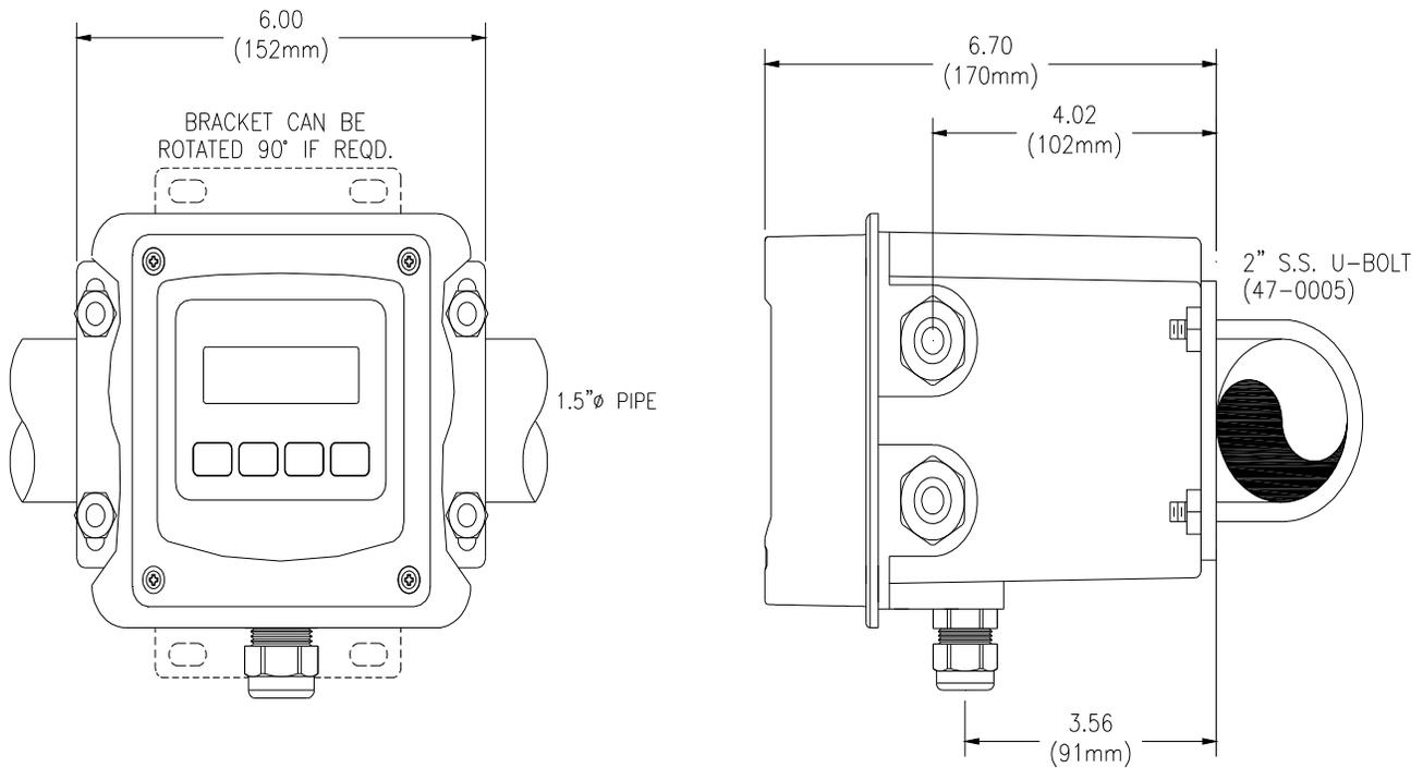
Figure 7 - Pipe Mounting Diagram
