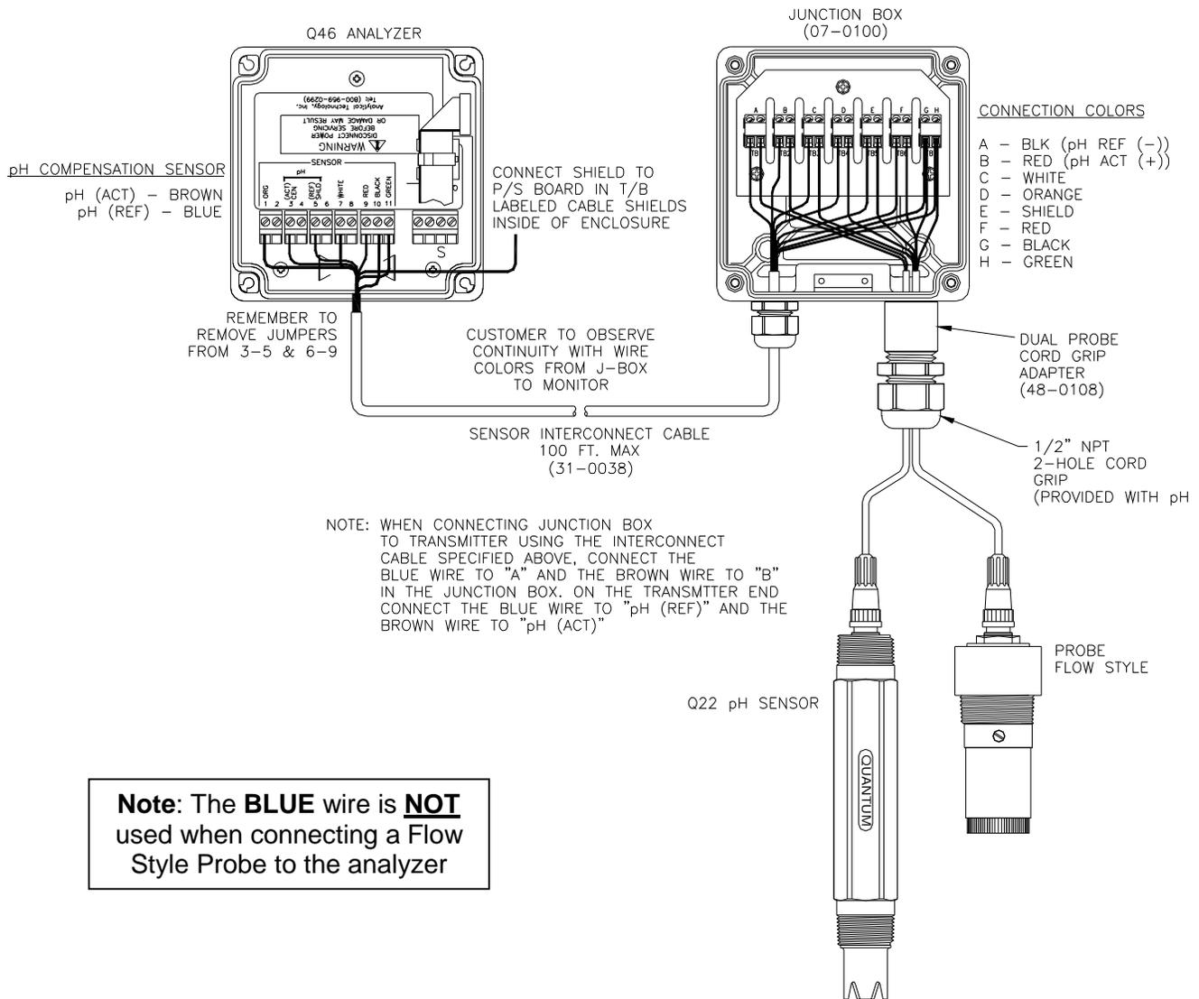
Figure 20 - Junction Box Wiring w/Optional pH Sensor
