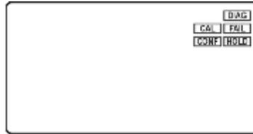
**HOLD** The HOLD icon indicates that the current output of the analyzer has been put into output hold. In this case, the output is locked to the last input value measured when the HOLD function was entered. HOLD values are retained even if the unit power is cycled.
