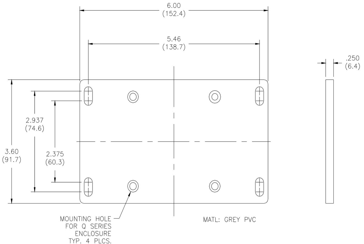
**Figure 5 - Wall or Pipe Mount Bracket**
