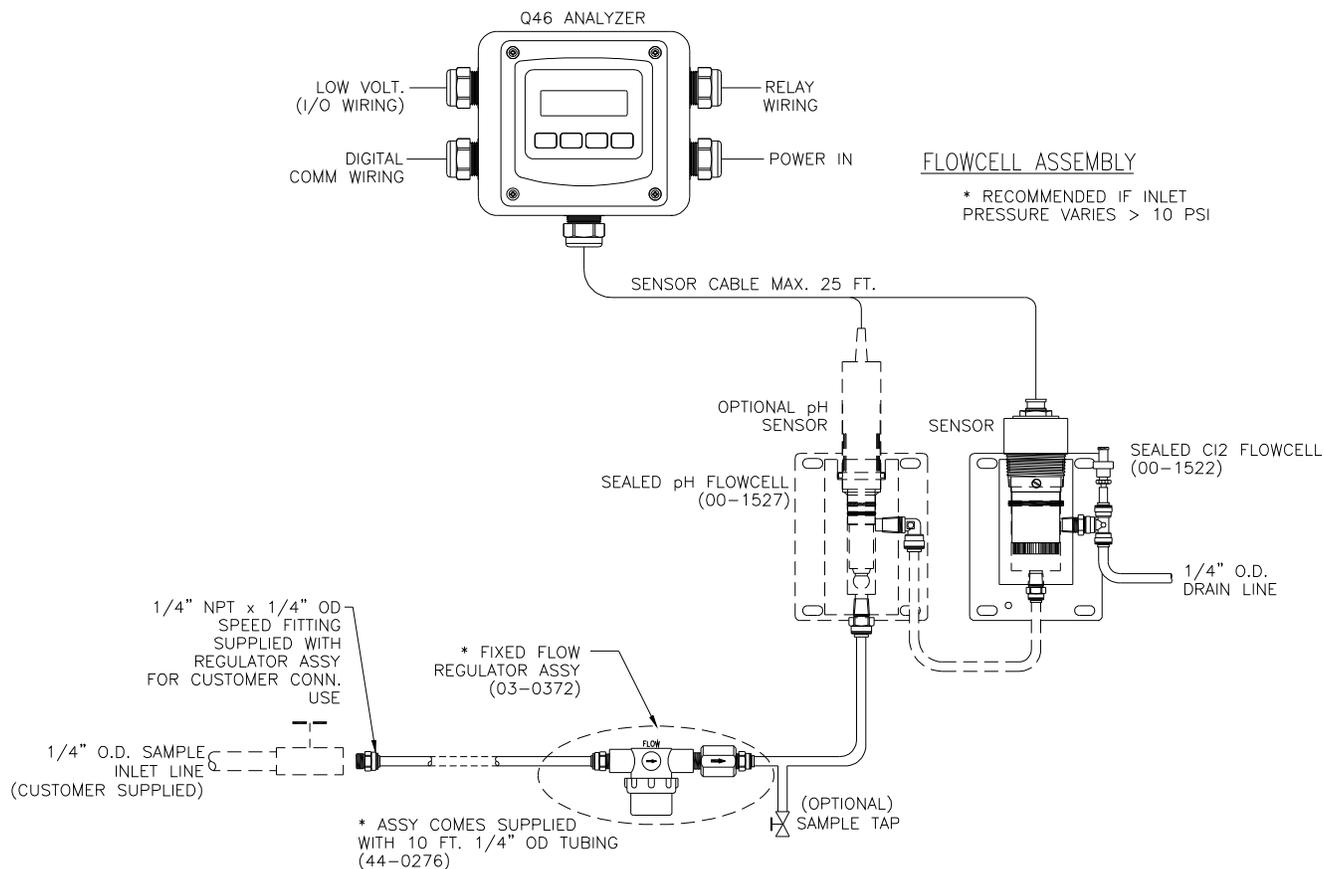
**Figure 3 - Sealed Flowcell Assemblies with Flow Control**
