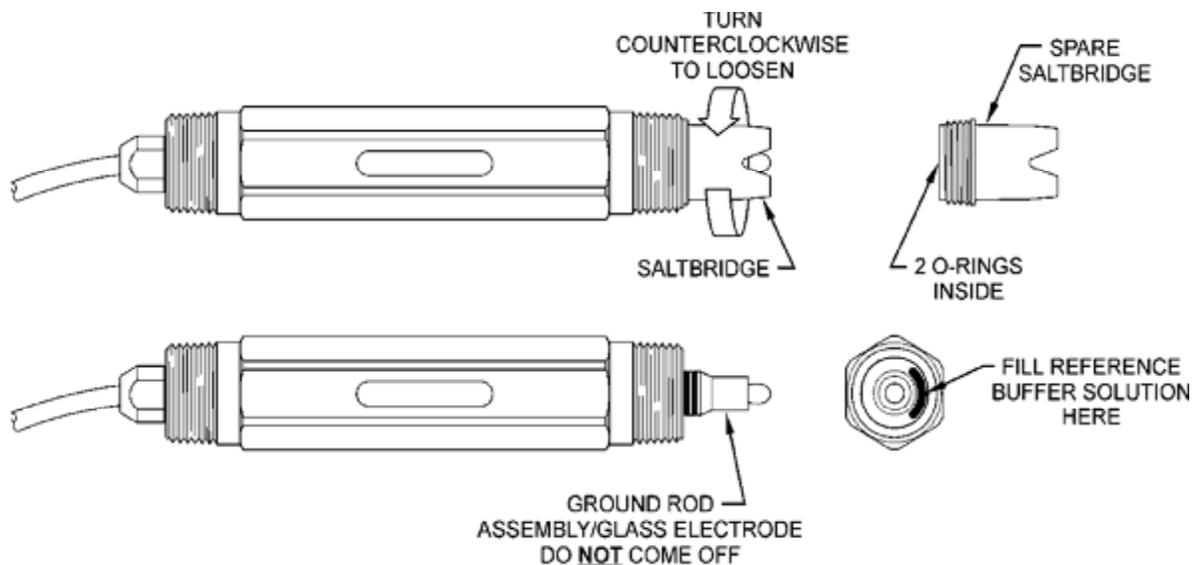
**Figure 28 - Replacing Saltbridge and Reference Buffer**
