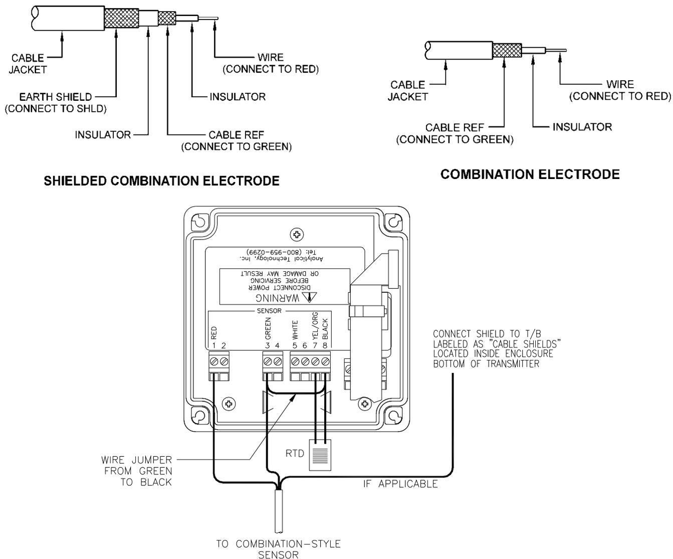
Figure 26 – OEM Sensor Connections, Combination Electrodes
