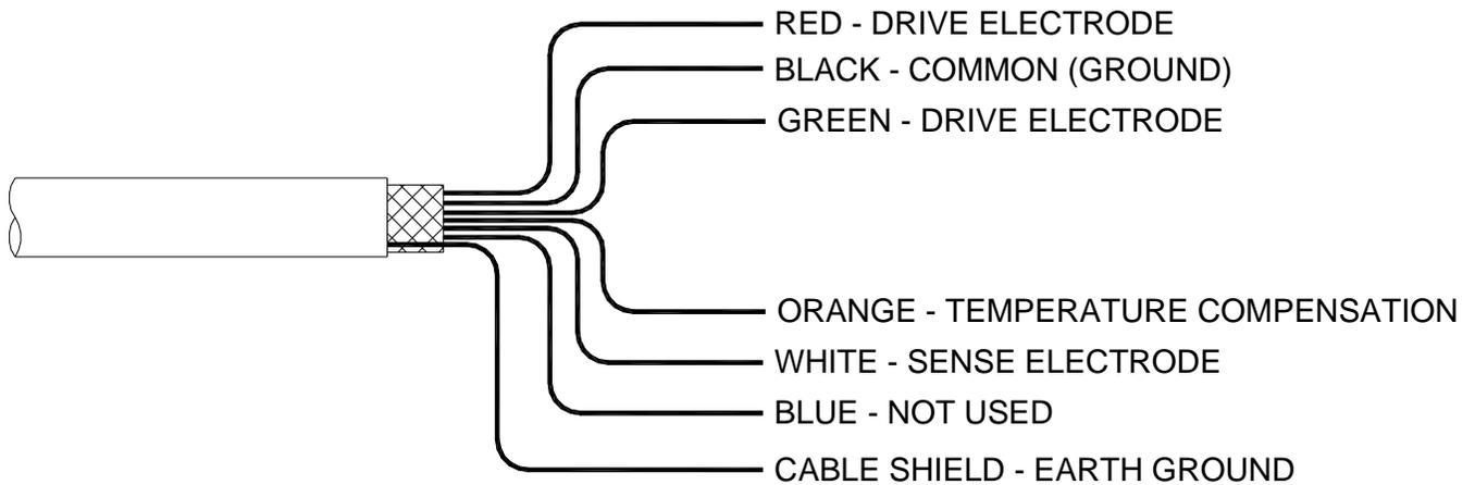
*Figure 22 - Detachable Single Shielded Cable, Model Q25P*
