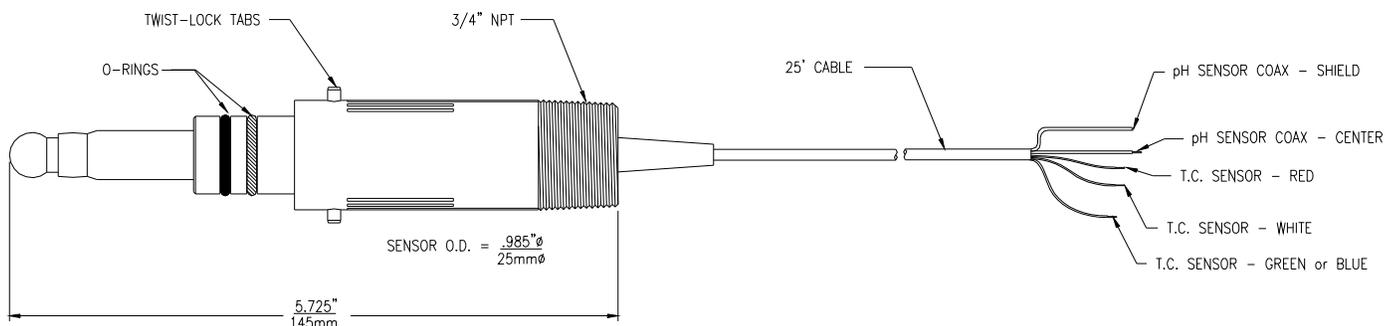
Figure 12 - (63-0013) Combination pH Sensor, Flow Type
