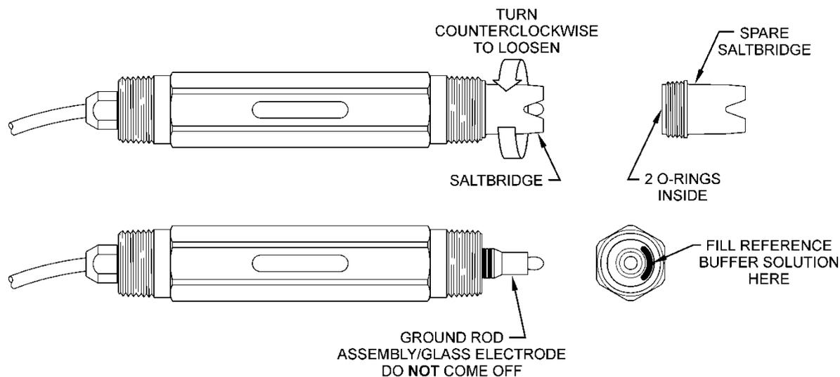
**Figure 36 - Replacing the Saltbridge and Reference Buffer**
