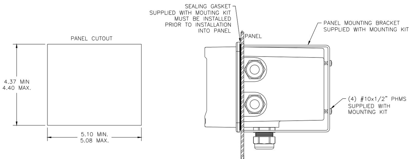
**Figure 5 - 115/230 VAC Panel Mount & Cut-out**
