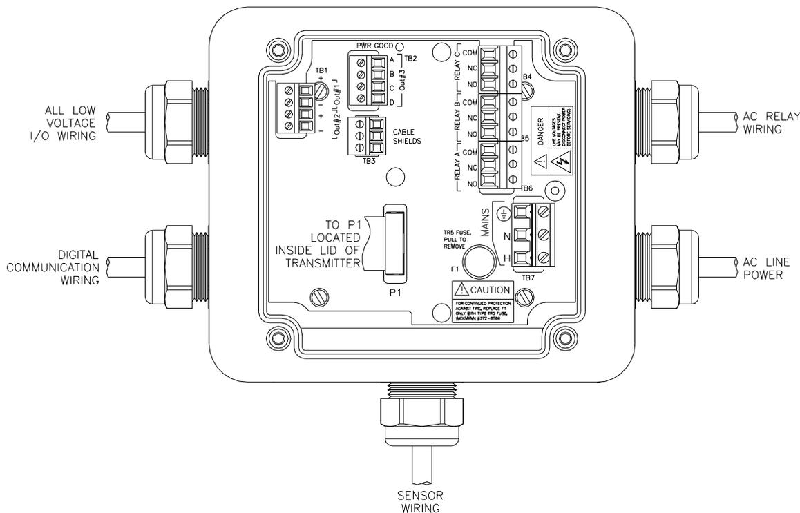
**Figure 17 – Q46 Connections**
