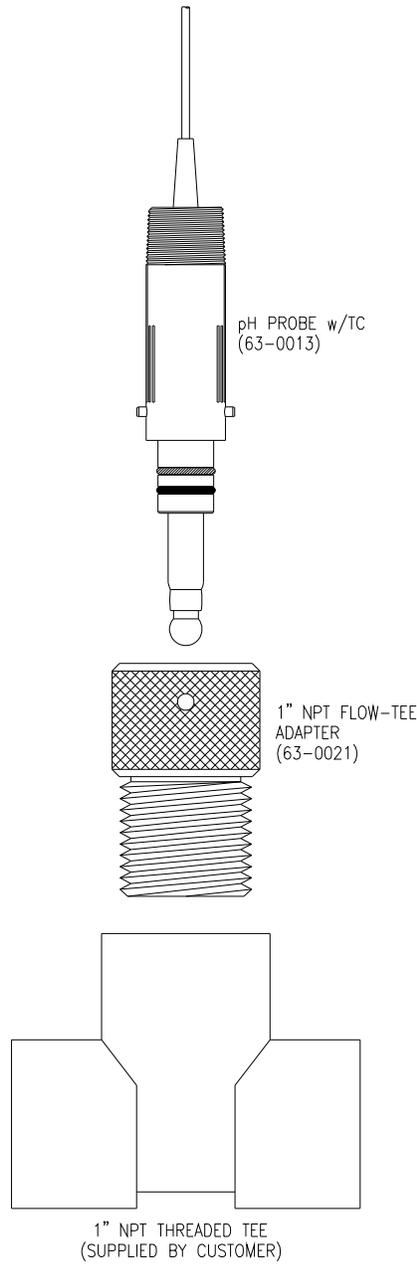
**Figure 15 - Twist-Lock Flow Tee**
