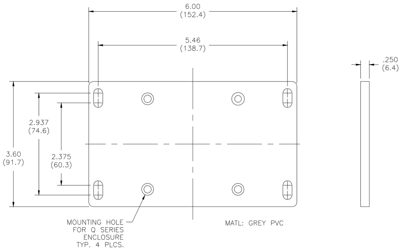
**Figure 2 - Wall or Pipe Mounting Bracket**
