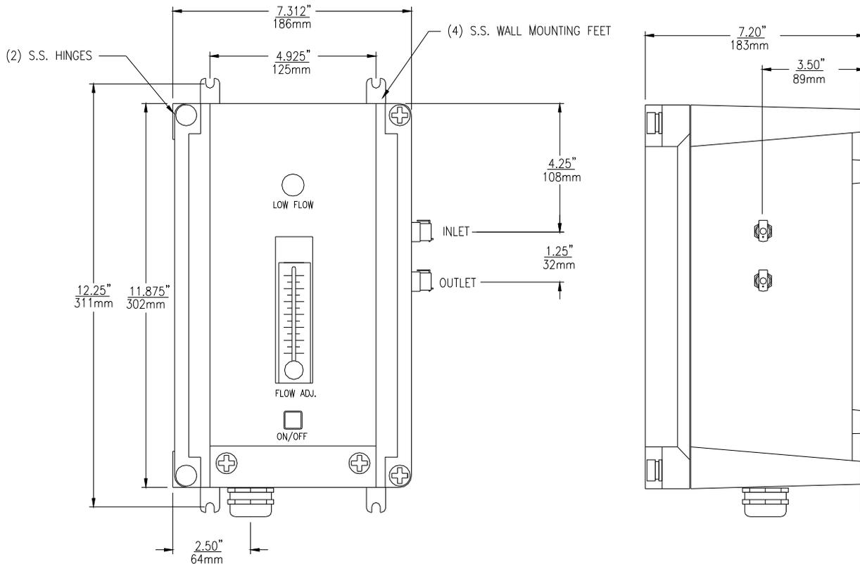
**Figure 2 - Sampling System Enclosure Dimensions (ATI-0228)**
