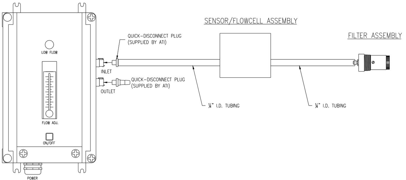
**Figure 1 - Sampling System General Arrangement (ATI-0229)**
