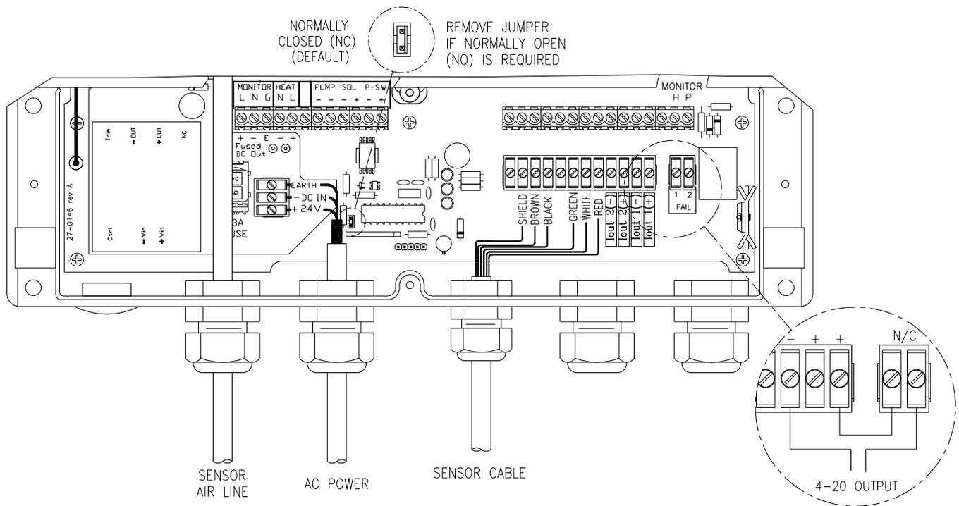
**Figure 14 - Cleaner Failure & Jumper Map Config**
