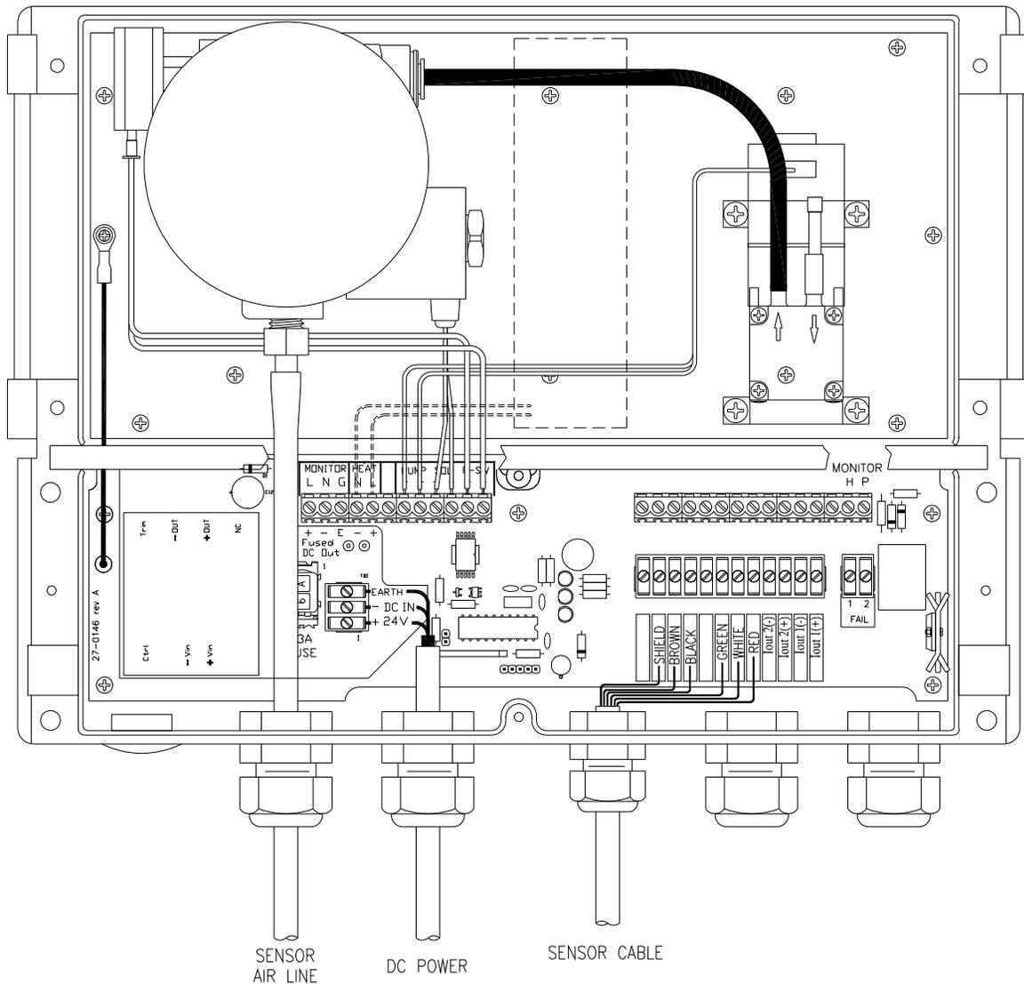
**Figure 6 - D.O. Monitor Electrical Connections**
