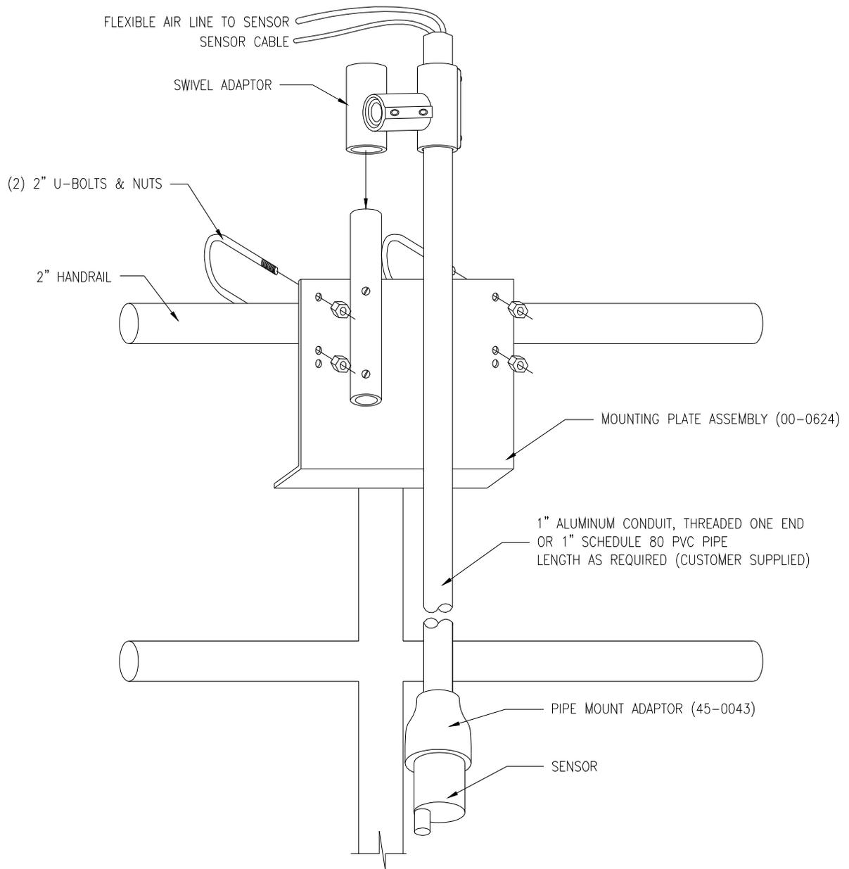
**Figure 5 - Mounting Assembly Detail**
