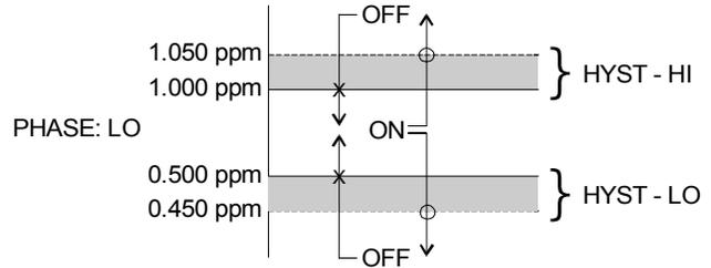
When value falls to  $\leq 0.500$  ppm, relay closes, until rises back to  $\geq 0.550$  ppm.
