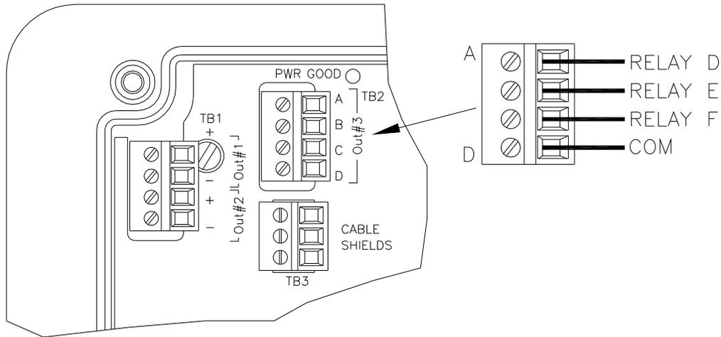
**Figure 12 - Low Power Relay Connections**
