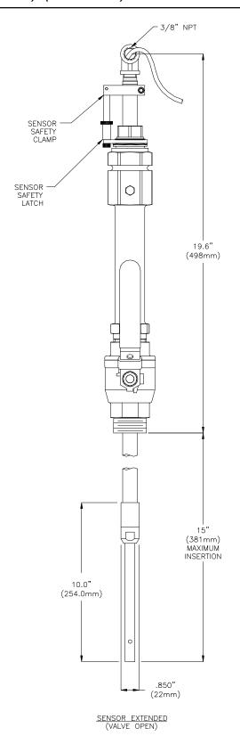
NOTE: Sensor is not part of (07-0203) insertion assembly
