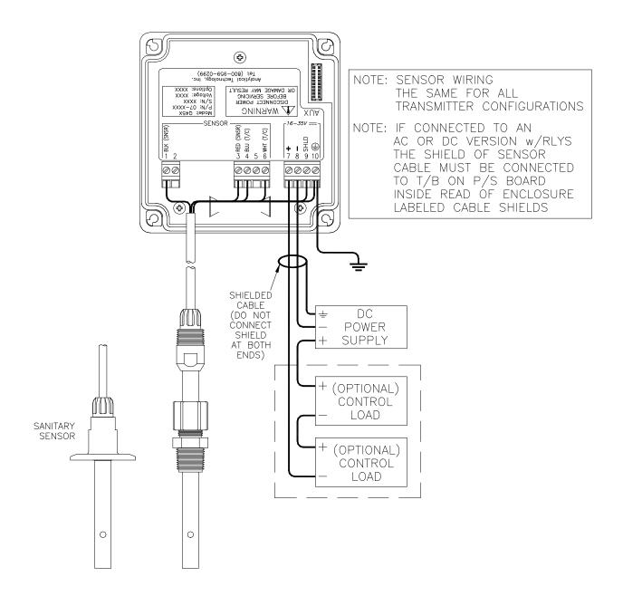
NOTES: 1. Voltage between Terminals 7 and 8 MUST be between 16 and 35 VDC.
