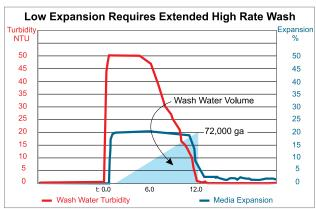
Insufficient media expansion extends the time required to purge turbidity from the filter and uses more wash water even at a reduced flow rate. Poor media expansion can also result in turbidity producing material remaining attached to media grains and not releasing in the wash
