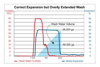
This filter was backwashed with a good rate of expansion and was clean with only six minutes of High Rate Wash – as indicated by Backwash Turbidity of 15 NTU. The operator did not have the benefit of a continuous, in-filter turbidity measurement and continued the high rate wash for an additional six minutes at a cost of an additional 48,000 gallons of wash water and no increase in cleaning effect.
