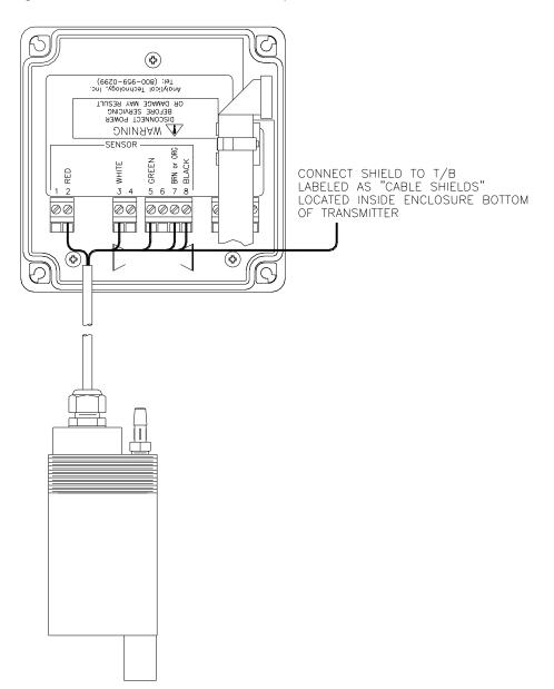
Figure 10 - Sensor Wiring
