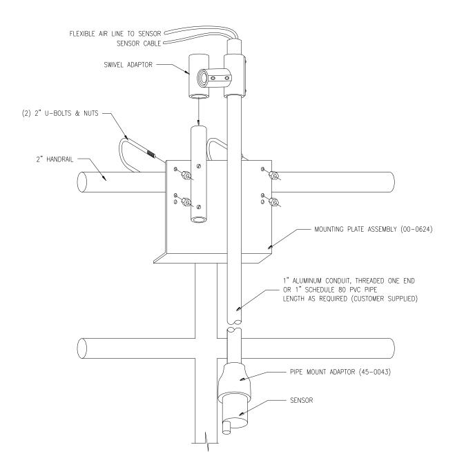
Figure 7 - Sensor Mounting Detail
