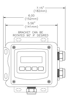
Figure 3 - Wall Mount Analyzer Dimensions
