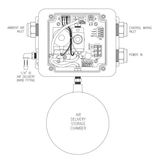
Figure 9 - Q-Blast Connections
