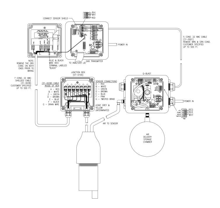
Figure 12 - Q-blast Connections w/Optional J-Box
