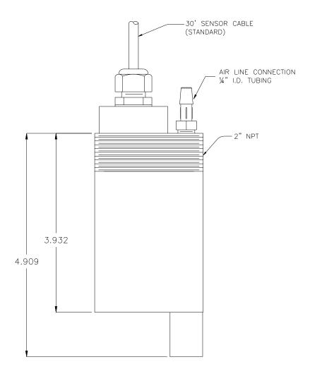
Figure 13 - Submersible D.O. Sensor Assy
