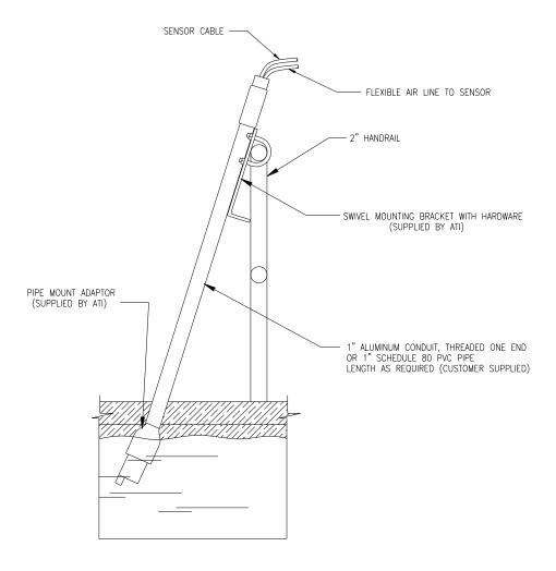
Figure 6 -Sensor Mounting Assembly
