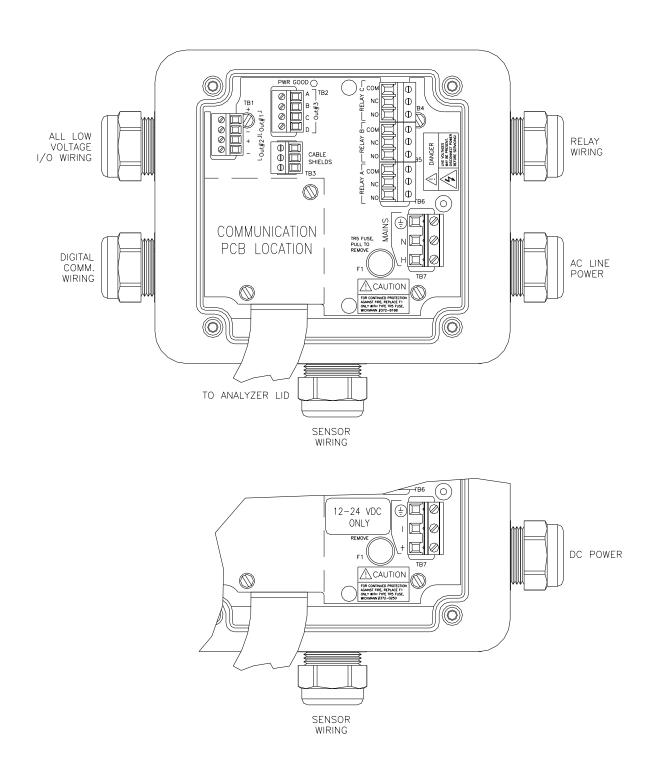
Figure 8 - Q46D Connections
