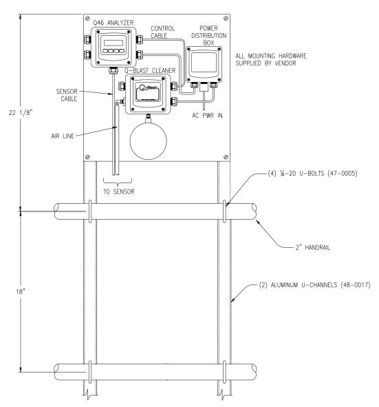
Figure 5 - Handrail Mounting Assembly
