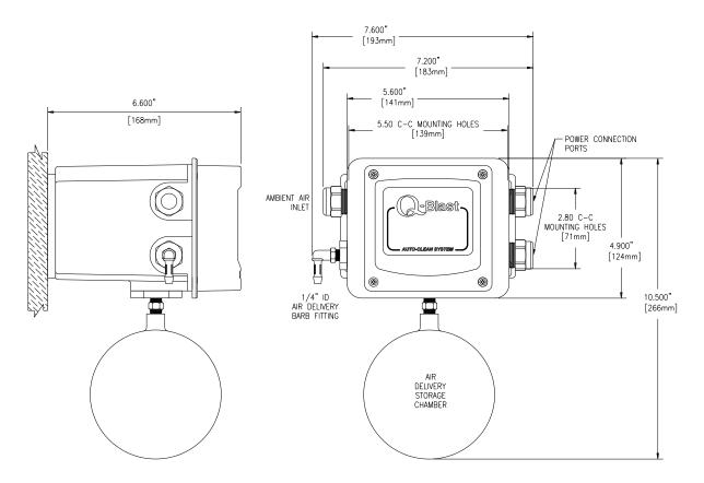
Figure 4 - Cleaner Enclosure Dimensions
