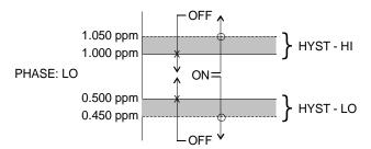
When value falls to  $\leq$  0.500 ppm, relay closes, until rises back to  $\geq$  0.550 ppm.
