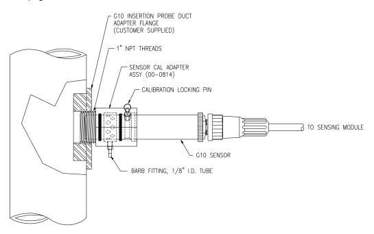
Figure 12 - Duct Mount Sensor Calibration (ATI-0299)
