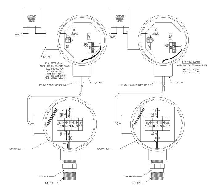
Figure 8 - Electrical Connections - C10 Dual Condulet Sensors (ATI-0101)
