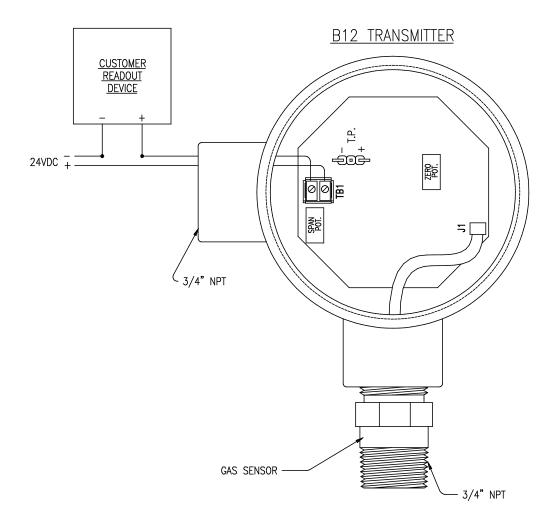
Figure 7 - Electrical Connections - Integral C10 Sensor
