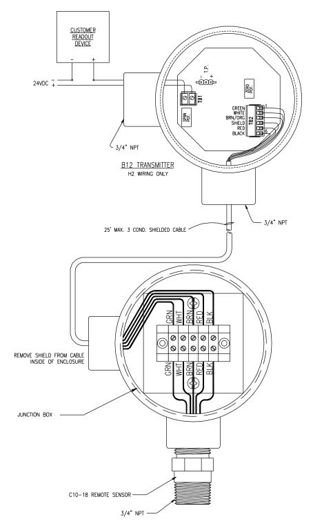
Figure 9 - Elect Connections - CV10-18 Only Dual Condulet Sensors (ATI-0101)
