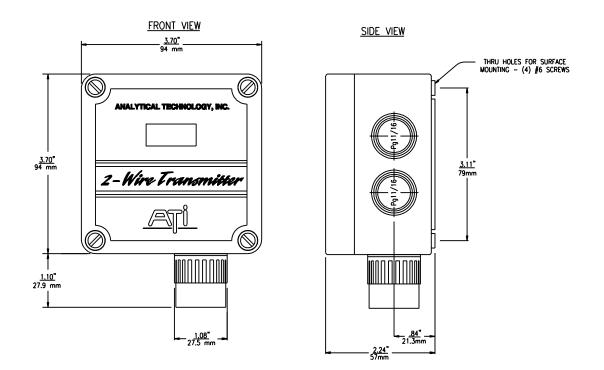
Figure 1 - Series B12 Nema 4X Transmitter Dinensions
