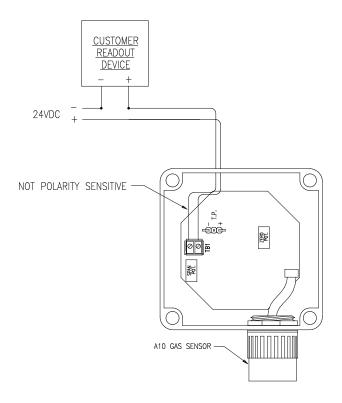
Figure 5 - Electrical Connections - Standard System
