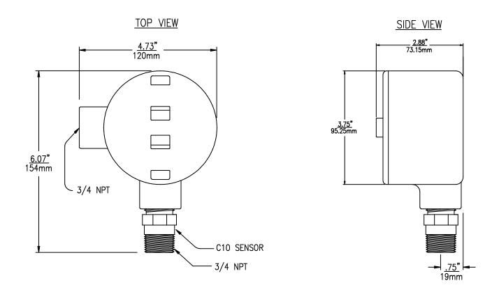
Figure 2 - Series B12 Explosion-Proof Transmitter Dimensions
