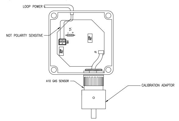
Figure 10 - Transmitter Controls & Test Points
