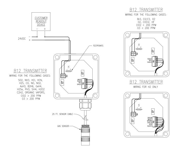
Figure 6 - Electrical Connections - Remote A10 Sensor - (ATI-0147)
