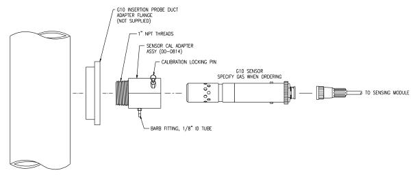
Figure 4 - Duct Mount Sensor Installation (ATI-0298)
