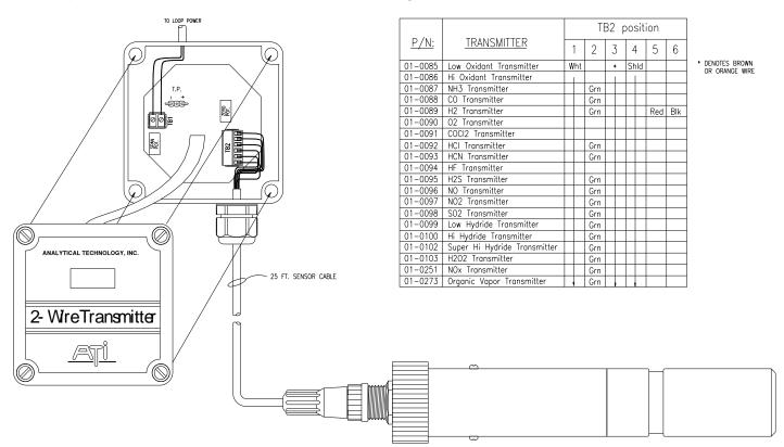
NOTE: All conductors on cable only used on H2 sensors only, the RED and BLK conductors can be removed from cable for all other gas applications.
