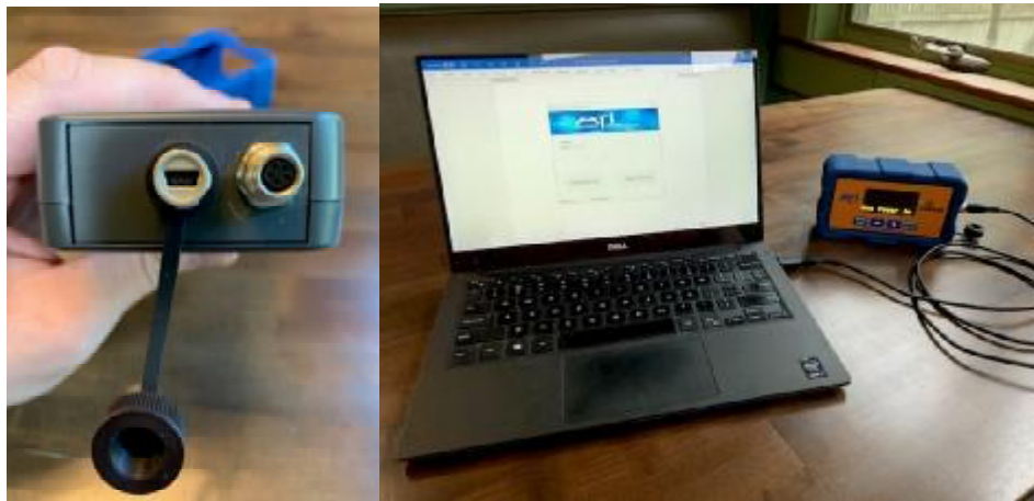
Figure 11 – Connecting Q51/MetriNet to Windows PC via USB
