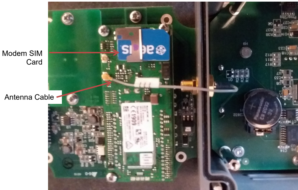
Figure 24 – MetriNet Cellular Modem Board with SIM Card
