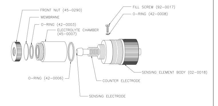
Figure 17 - PAA Sensor Assembly
