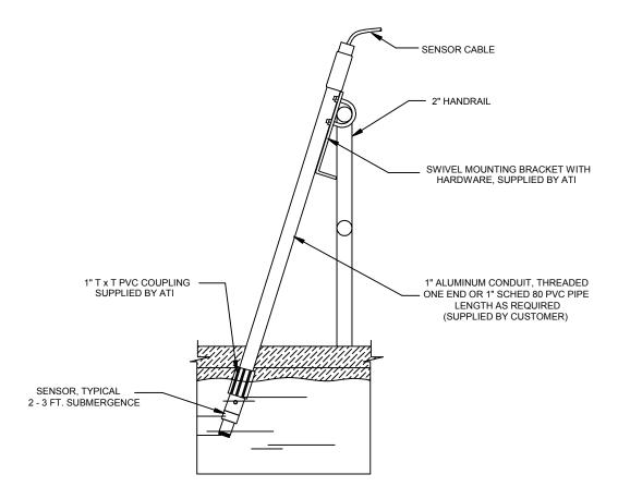
Figure 11 - Submersible Sensor Mounting Assembly
