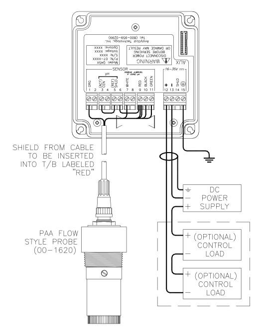
Figure 12 - Loop Power Sensor Connection
