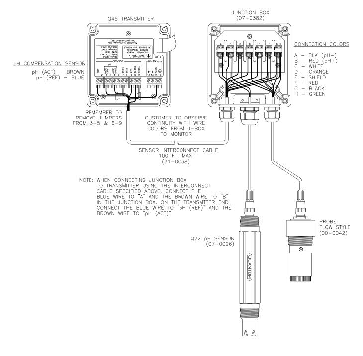
Figure 16 - Optional pH Sensor Connection w/Junction Box
