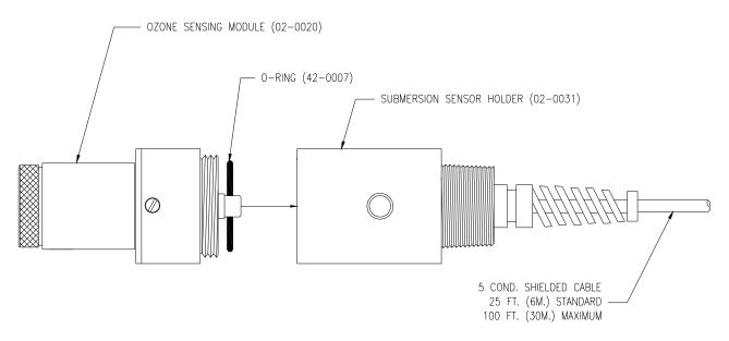
Figure 18 - Submersible PAA Sensor Assembly
