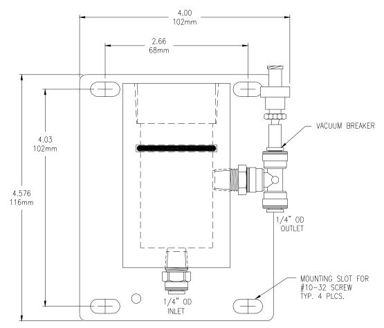
Figure 9 - Sealed Flowcell Details
