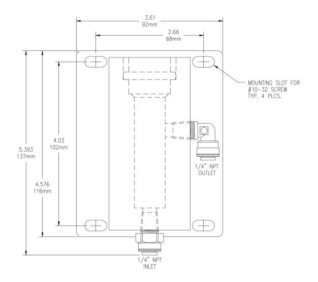
Figure 10 - Sealed pH Flowcell Details
