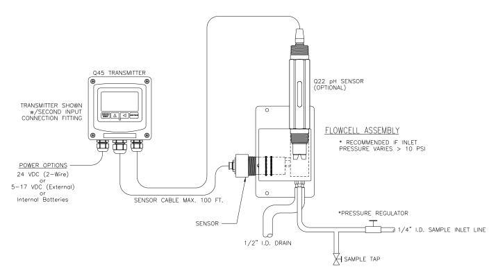
Figure 1 - Typical Monitoring System
