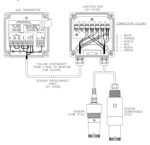
Figure 14 - Junction Box Interconnect Wiring
