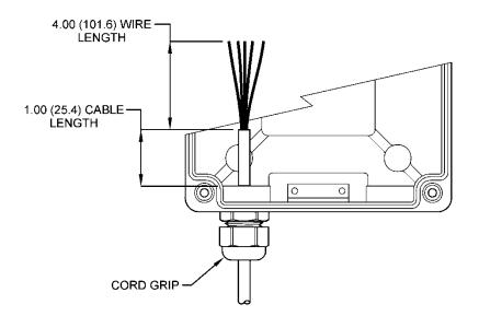
Figure 13 - Sensor Cable Preparation
