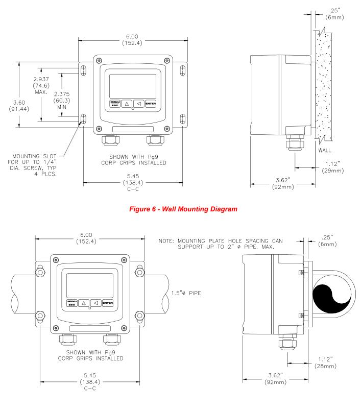
Figure 7 - Pipe Mounting Diagram
