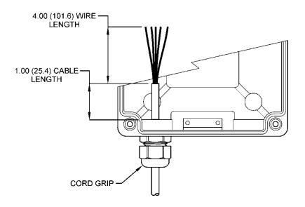
Figure 13 - Sensor Cable Preparation
