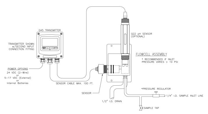
Figure 1 - Typical Chlorine Dioxide Monitoring System
