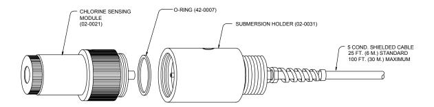
Figure 18 - Submersible Chlorine Dioxide Sensor Assembly
