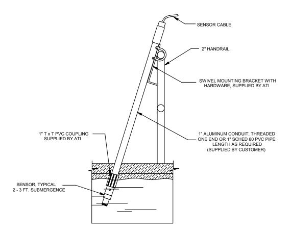
Figure 11 - Submersible Sensor Mounting Assembly
