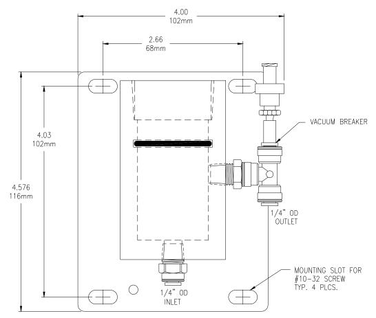
Figure 9 - Sealed Flowcell Details
