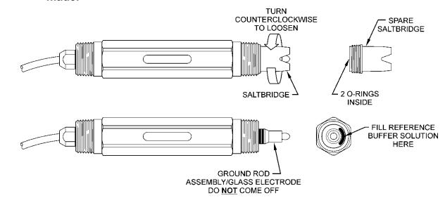
Figure 23 - Replacing the Saltbridge and Reference Buffer
