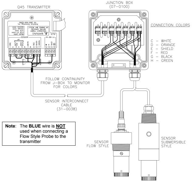
Figure 14 - Junction Box Interconnect Wiring
