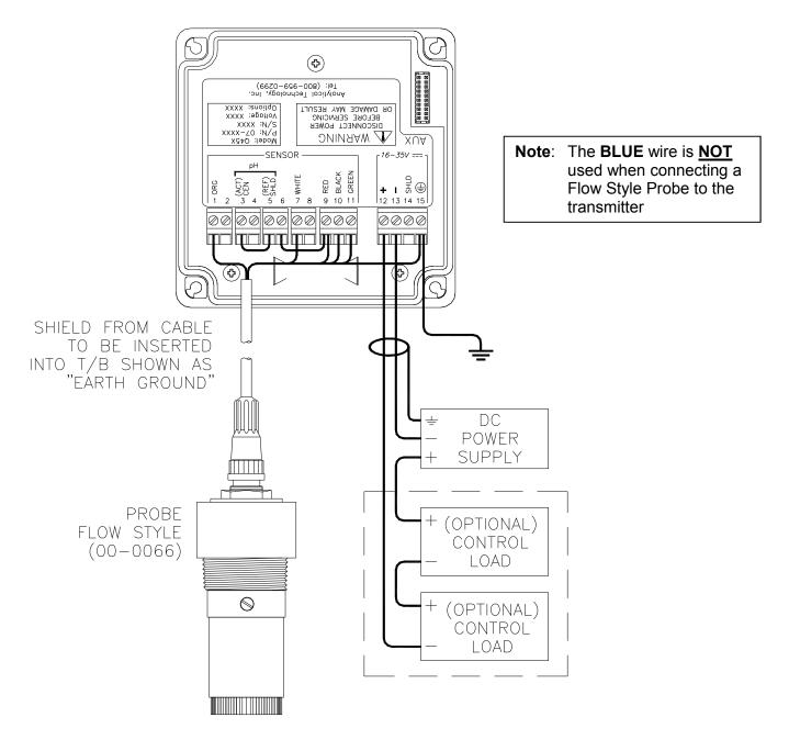
Figure 12 - Loop Power Sensor Connection
