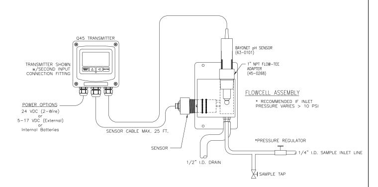
Figure 2 - Monitoring System w/Bayonet style pH Sensor
