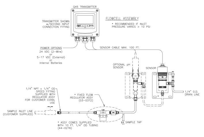
Figure 3 - Sealed Flowcell Assemblies w/Flow Control
