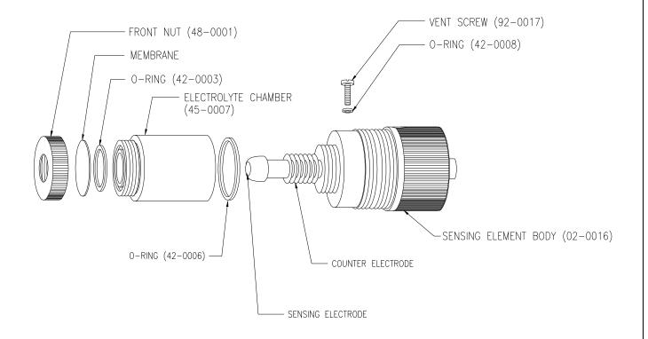
Figure 17 - Chlorine Dioxide Sensor Assembly
