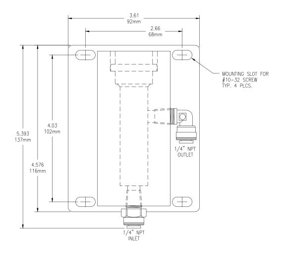
Figure 10 - Sealed pH Flowcell Details
