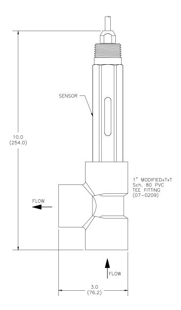
Figure 6 - Flow Through Tee Mount
