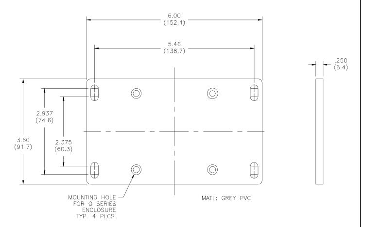
Figure 2 - Wall or Pipe Mount Bracket
