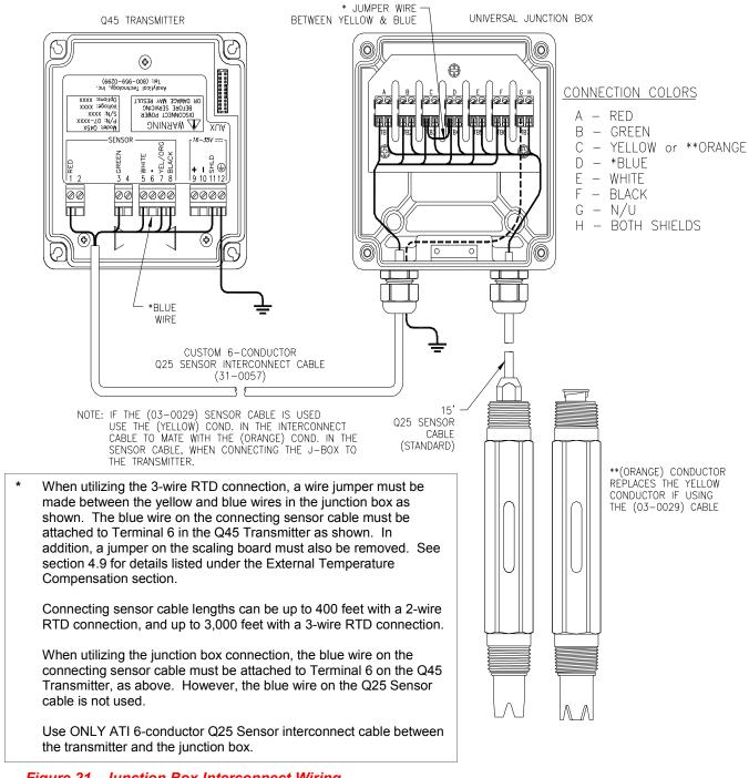
Figure 21 - Junction Box Interconnect Wiring
