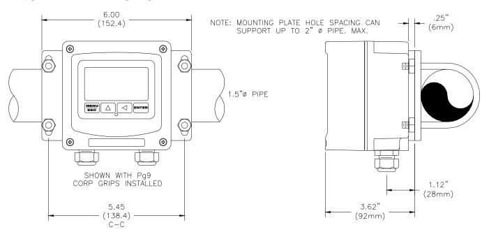
Figure 4 - Pipe Mounting Diagram
