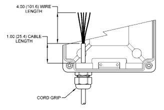
Figure 20 - Sensor Cable Preparation
