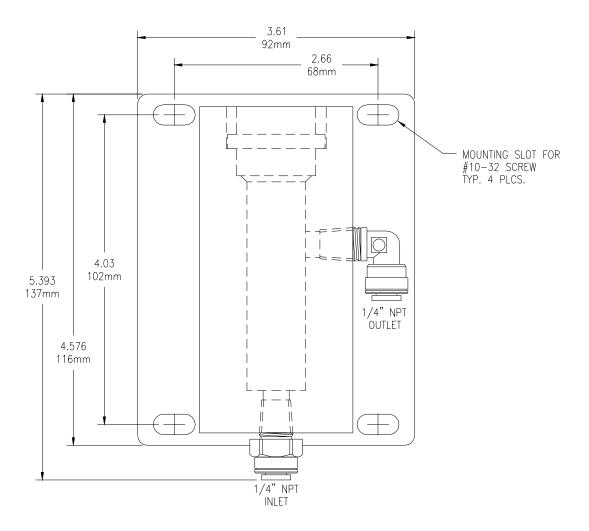
Figure 14 - Sealed Flowcell Details
