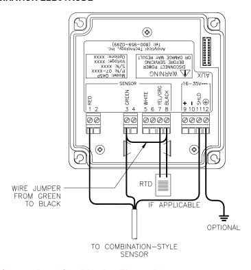
Figure 22 - Sensor Connections, Combination Electrodes
