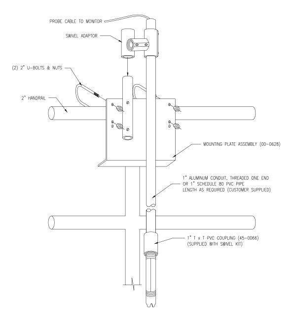
Figure 9 - Sensor Submersion Mount
