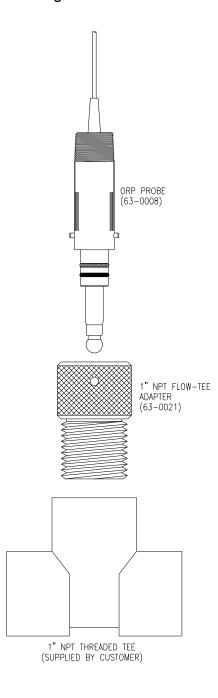
Figure 15 - Twist-Lock Tee
