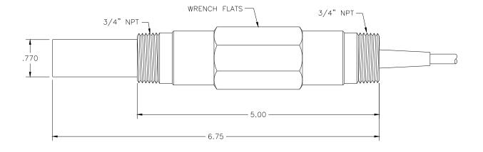
Figure 13 - (63-0023) Combination ORP Sensor - Submersion
