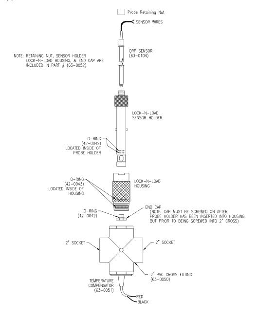
Figure 16 - Lock-n-Load Sensor Exploded View
