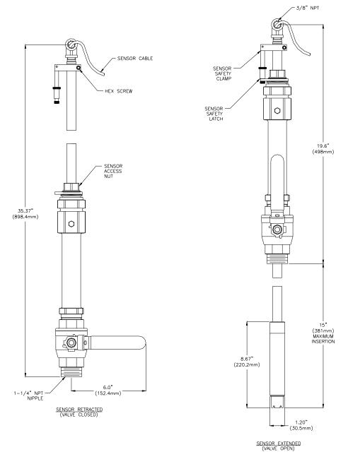
Figure 10 - S.S. Sensor Insertion Mount
