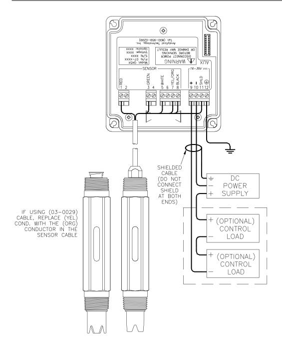
Figure 17 - Loop Power Wiring Diagram
