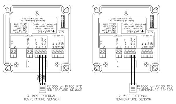
Figure 24 - External Temperature Compensation Figure
