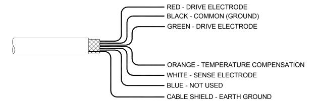
Figure 19 - Detachable Single Shielded Cable, Q25R
