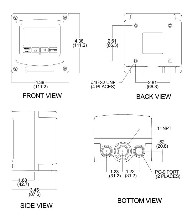
Figure 1 - Q45 Enclosure Dimensions
