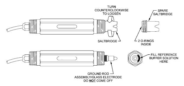
Figure 28 - Replacing the Saltbridge and Reference Buffer
