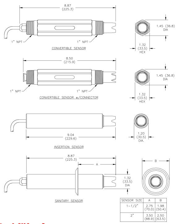
Figure 5 - Q25 Sensor Types
