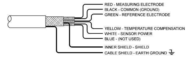
Figure 18 - Cable Description, Model Q25
