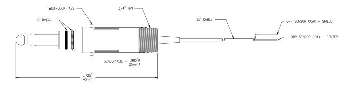
Figure 12 - (63-0008) Comb. ORP Sensor - Flow
