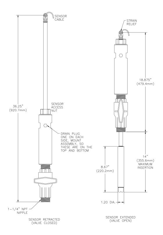
Figure 11 - CPVC Sensor Insertion Mount
