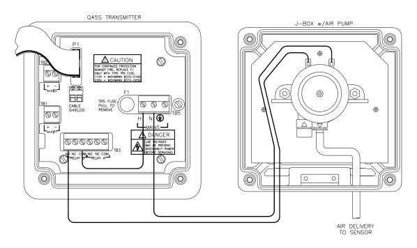
Figure 12 - Pump Interconnect Connection
