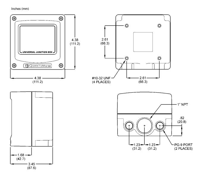
Figure 8 – Air Pump Enclosure Specifications
