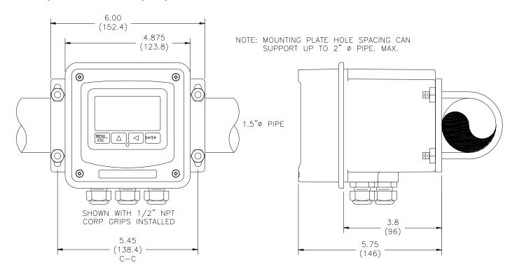
Figure 6 - Pipe Mounting Diagram
