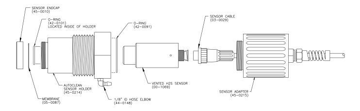
Figure 10 - Duct Insertion Sensor Holder Exploded View
