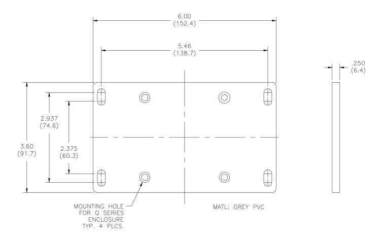
Figure 4 - Wall or Pipe mount Bracket
