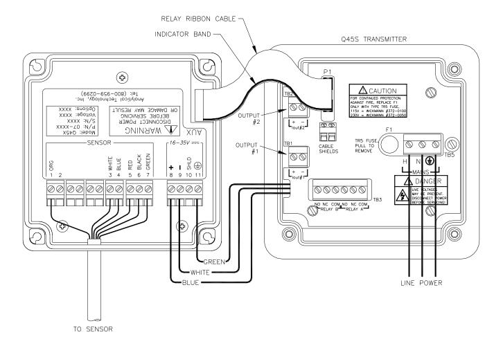
Figure 14 - Sensor Connection
