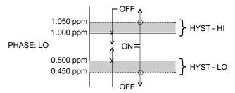
When value falls to < 0.500 ppm, relay closes, until rises back to > 0.550 ppm. When value rises to ≥ 0.500 ppm, relay closes, until value falls back to < 0.450 ppm.
