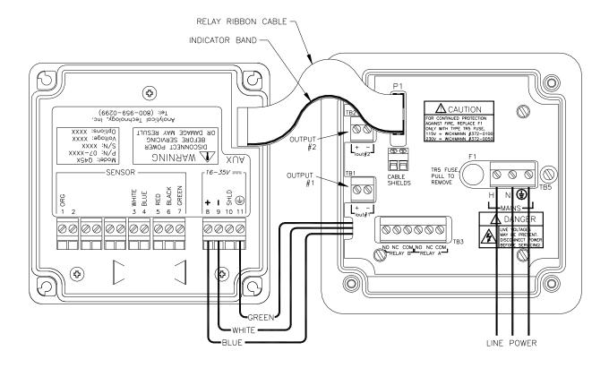
Figure 11 - Line Power Connection
