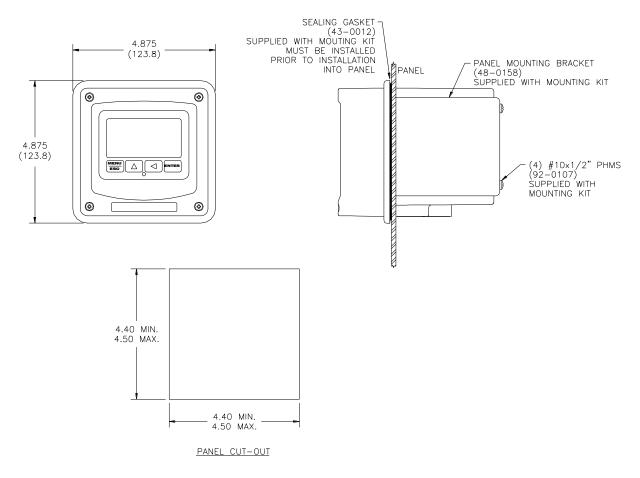
Figure 7 - Panel Mount Cut-Out
