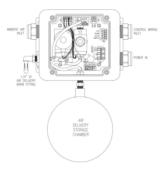
Figure 9 - Q-blast Connections
