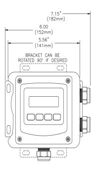
Figure 3 - Wall Mount Analyzer Dimensions
