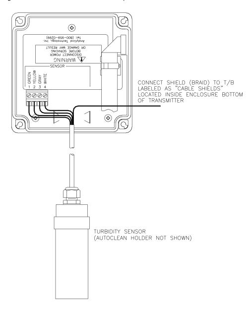
Figure 10 - Turbidity Sensor Connection
