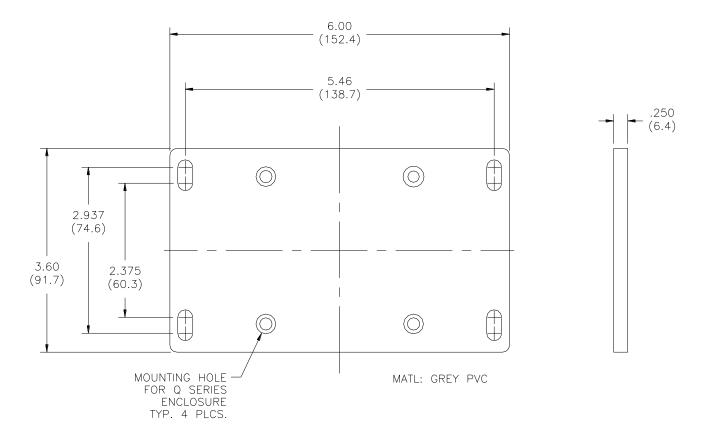
Figure 2 - Wall/Pipe Mount Bracket
