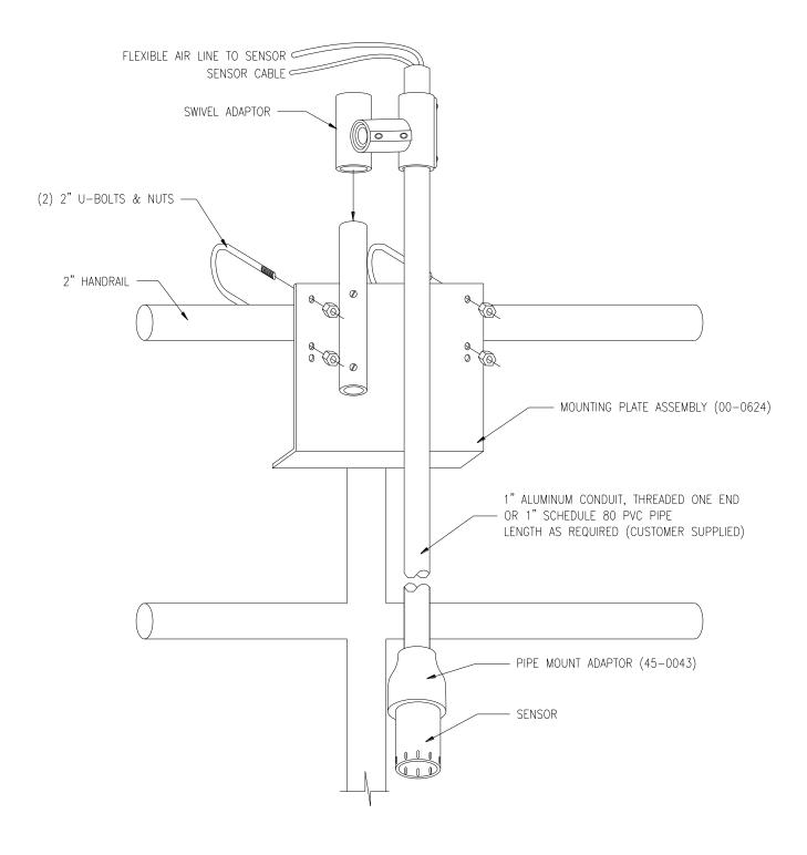
Figure 7 - Sensor Mounting Detail
