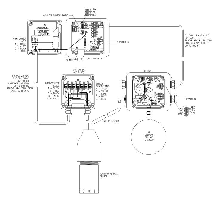
Figure 12 - Q-Blast Connections w/Optional J-Box
