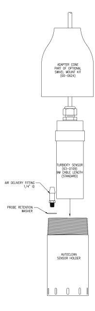
Figure 5 - Sensor Assembly
