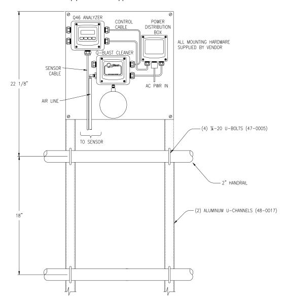
Figure 4 - Handrail Mounting Assembly
