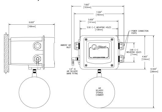
Figure 3 - Q-Blast Cleaner Dimensions
