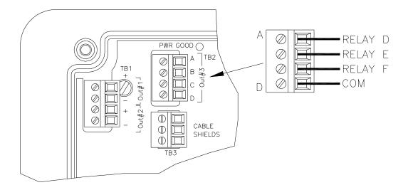
Figure 15 - Optional Relay Board Wiring
