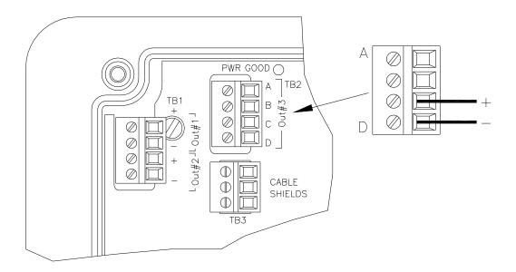
Figure 16 - Optional Analog Output Wiring
