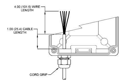
Figure 17 - Sensor Cable Preparation
