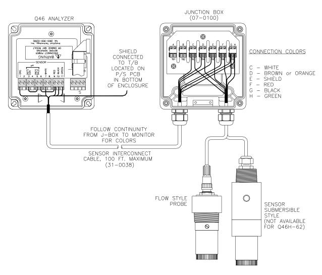
Figure 19 - Junction Box Interconnect Wiring
