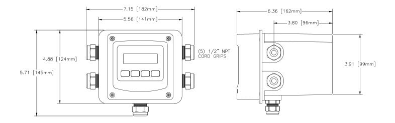
Figure 4 - Q46 Enclosure Dimensions
