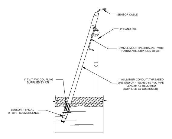
Figure 12 - Submersible Sensor Mounting Assembly
