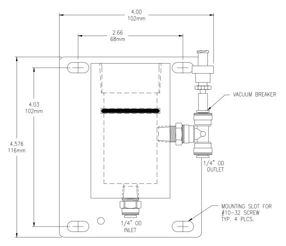
Figure 10 - Sealed Cl<sub>2</sub> Flowcell Details
