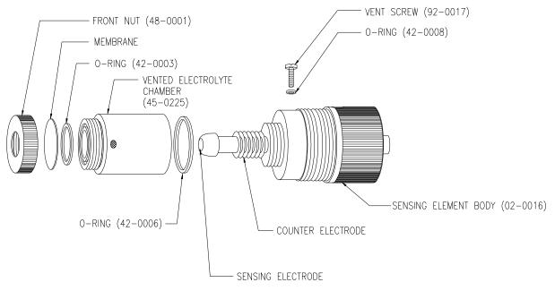
Figure 20 - Chlorine Sensor Assembly
