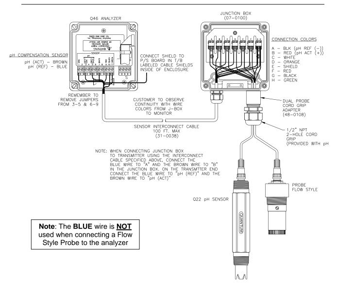
Figure 20 - Junction Box Wiring w/Optional pH Sensor
