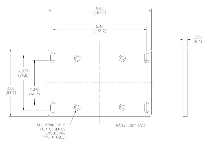
Figure 5 - Wall or Pipe Mount Bracket
