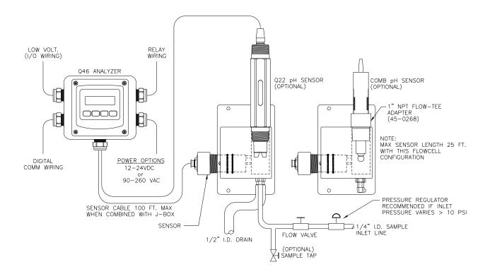
Figure 2 - Chlorine System w/Conventional pH Style Sensor
