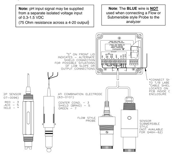
Figure 18 - Direct Sensor Connection
