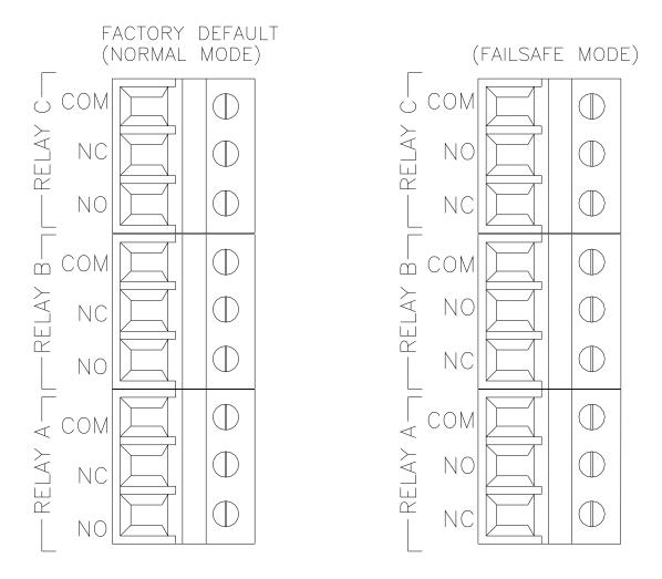
Figure 14 - Optional Relay Board Wiring
