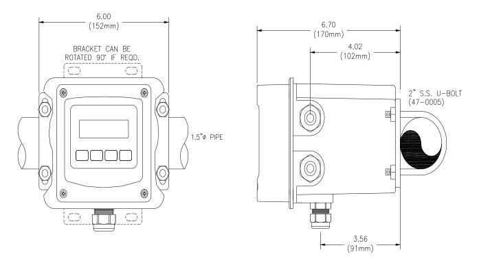
Figure 7 - Pipe Mounting Diagram
