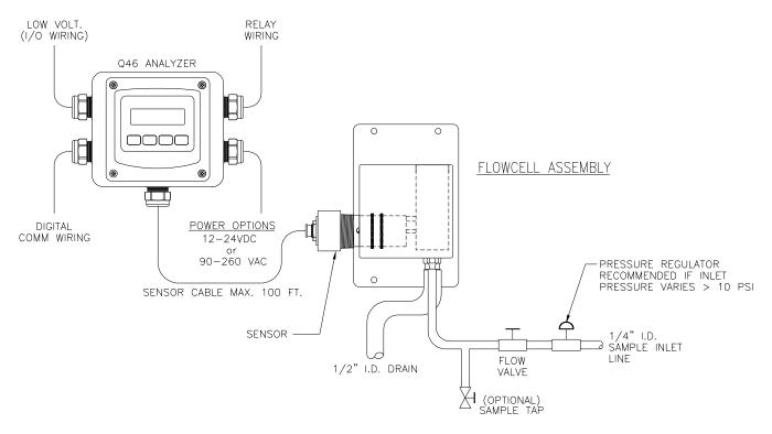
Figure 1 - Typical Chlorine Monitoring System
