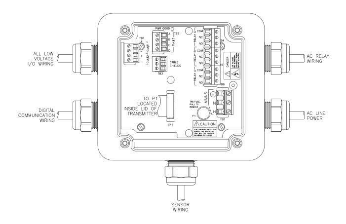
Figure 13 - Line Power Connection
