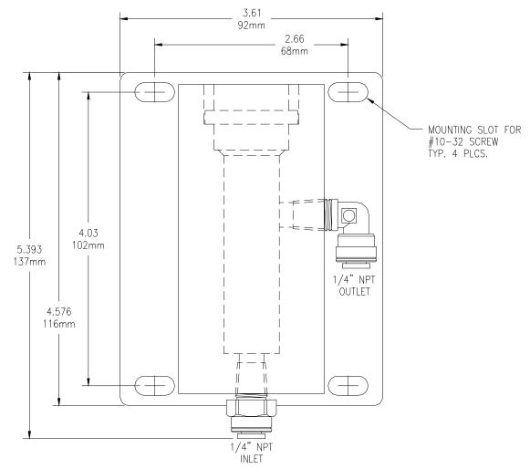
Figure 11 - Sealed pH Flowcell Details
