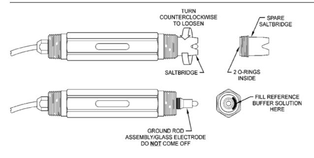
Figure 28 - Replacing Saltbridge and Reference Buffer
