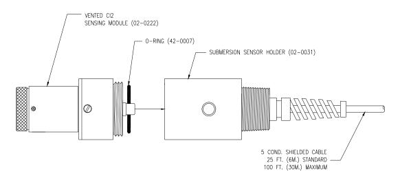
Figure 21 - Submersible Chlorine Sensor Assembly
