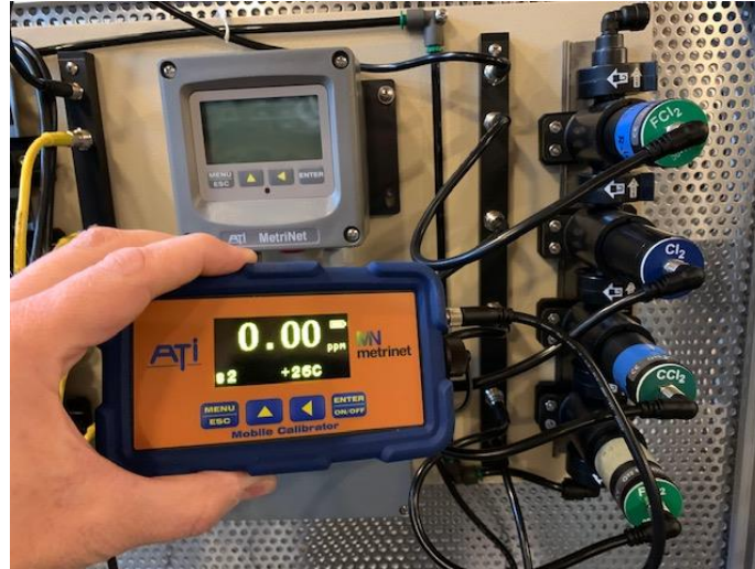
Figure 8 – Bus Operation of Several M-Node Sensors
