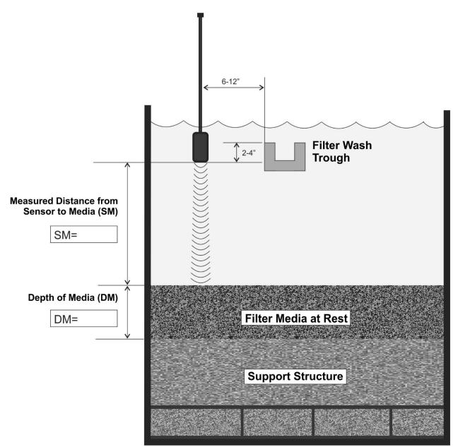
Figure 45: Installation Recommendations for Filter Applications
