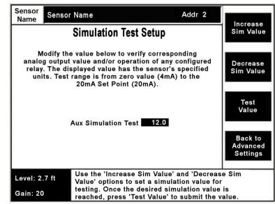
Figure 35: Aux Simulation Test Setup Screen
