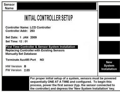
Figure 5: Initial Controller Setup
