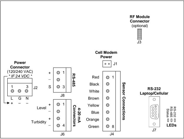
Figure 21: Connections for Power Supply
