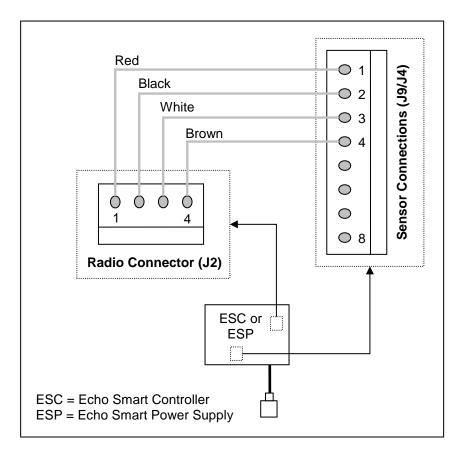
Figure 37: Connections for Wireless Radio Module (External)
