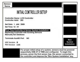
Change the Sensor Address to a unique value other than 1 and enter the correct parameters associated with the sensor on the Initial Sensor Setup screen – most importantly the Tank Depth, Zero Adjust, and 4-20mA Set Points (if being used). See Section 7.1 for help in determining correct values for Tank Depth and Zero Adjust. Press Sensor Setup Complete.
