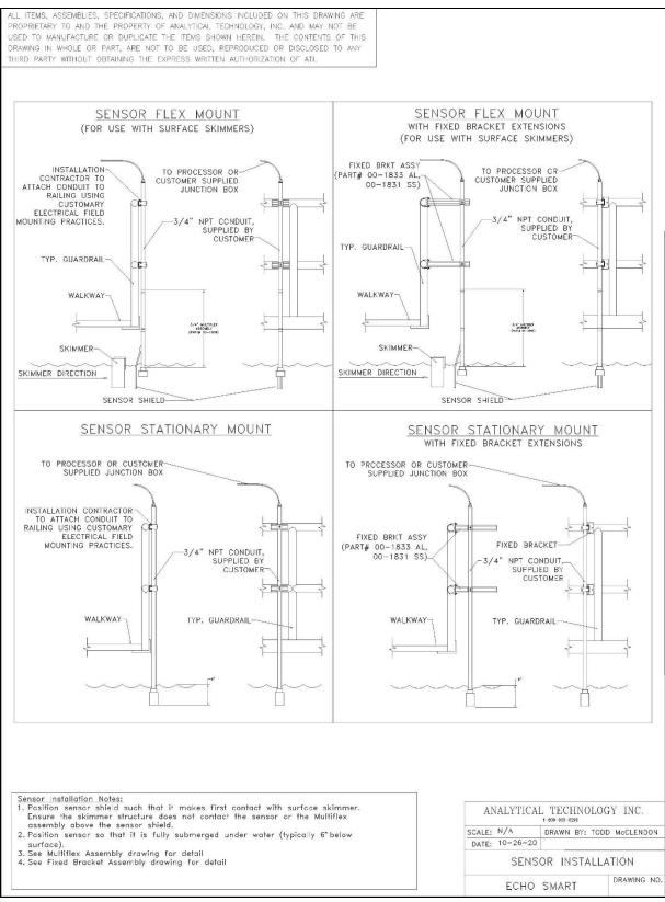
Figure 23: EchoSmart Sensor Installation Arrangements
