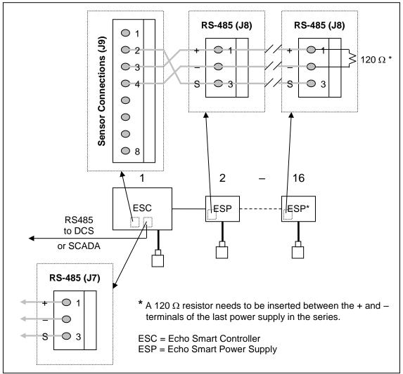
Figure 30: Single Wired Field Network
