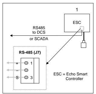
Figure 29: Controller with Single Sensor
