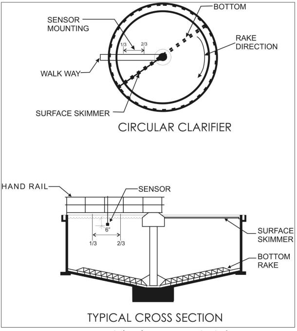
Figure 24: Typical 1/3 – 2/3 Location in Circular Clarifier
