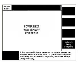
5. Repeat steps 3 and 4 for all sensors in the network, ensuring that each sensor has a unique Sensor Address. Once all have been setup, press *Network Setup Complete*.
