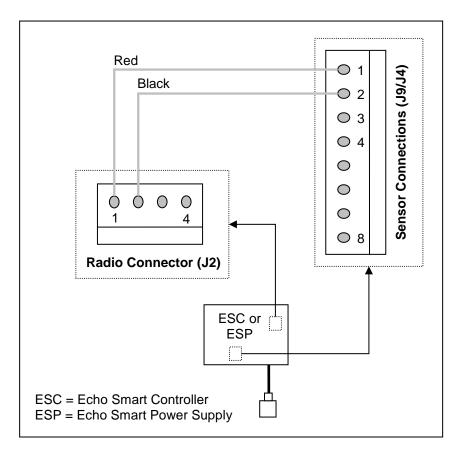
Figure 36: Connections for Wireless Radio Module (Internal)
