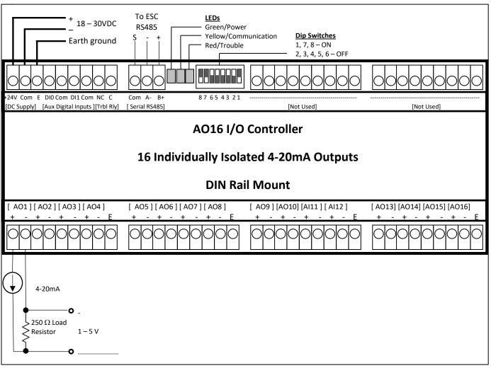
Figure 42: Analog Output Module Connections
