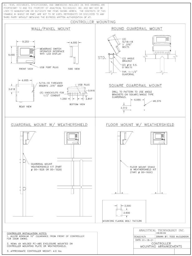
Figure 25: Controller Installation Drawing
