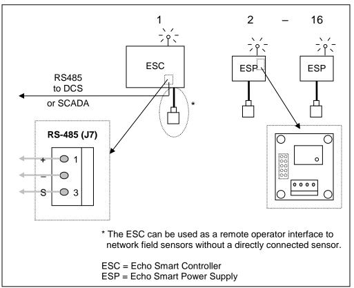
Figure 31: Single RF Field Network
