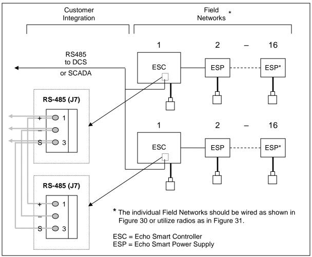
Figure 32: Integrated Wired Field Network
