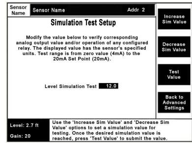
Figure 34: Level Simulation Test Setup Screen
