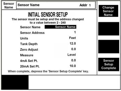
Figure 6: Initial Sensor Setup
