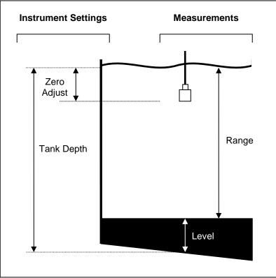
Figure 27: Tank Configuration
