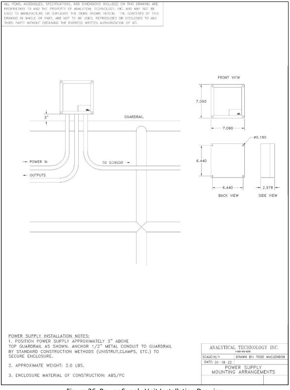
Figure 26: Power Supply Unit Installation Drawing
