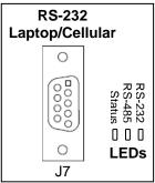
If the *Status* LED is on solid and the *RS-485* LED is not flashing, verify that the radio is seated properly and cycle power to determine if communication can be re-established.
