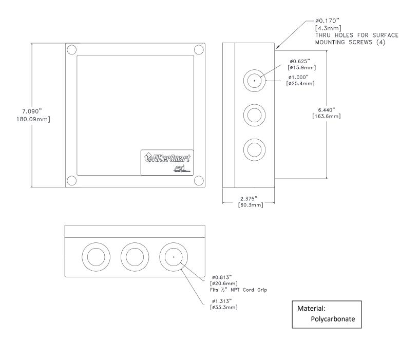
CAUTION: Be very careful when removing the knockouts on the enclosure. A small bladed screwdriver tapped firmly in the knockout recess is all that is necessary. Do not drive the screwdriver blade into the enclosure or it may strike the circuit board and cause component damage.
